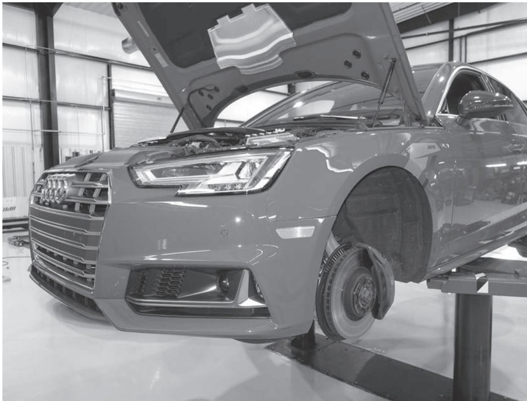
1) Place the vehicle securely on jack stands or on a lift, remove the front wheels, and raise the hood of the vehicle.
