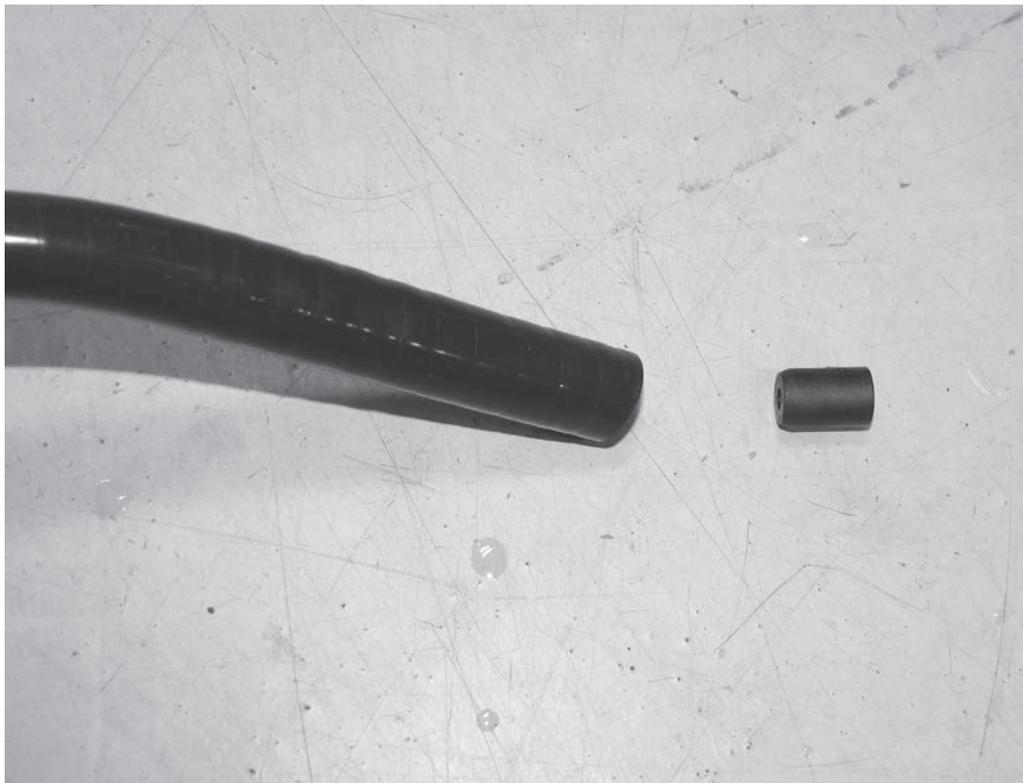
5) Install the one way check valve in the end of the APR hose that goes to the engine. Be sure to install the check valve in the same orientation as it was in the stock coolant hose.
