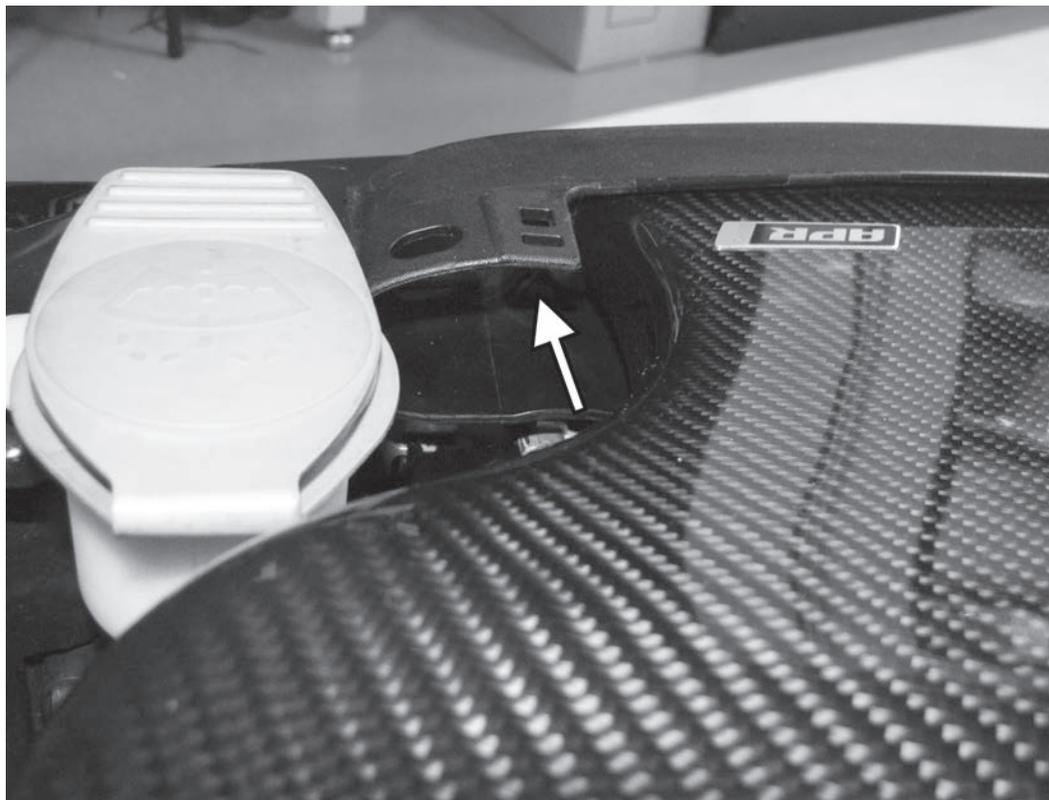
7) Carefully loosely place the APR intake back in the car. Connect the intake into the slot on the back side of the core support, and then slide the intake towards the right side of the car to lock it in place. Install the screw holding the APR intake to the back side of the radiator core support.
