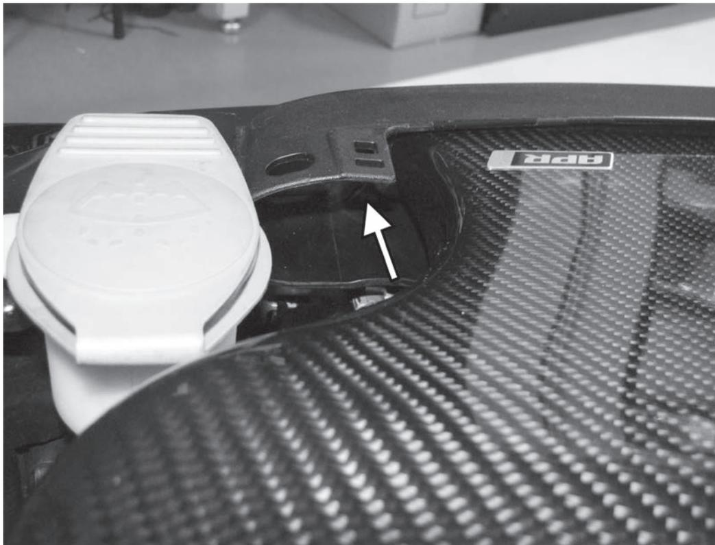
1) Once making sure the engine is cold, remove the cap from the factory coolant reservoir. Remove the screw holding the APR intake to the back side of the radiator core support. Slide the intake towards the left side of the car to separate it from the core support.
