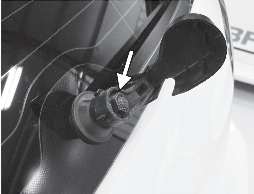
1) Carefully pry up the cover to the rear wiper by lifting the plastic cap from the left side of the wiper. Remove the 13mm nut holding the wiper in place.
