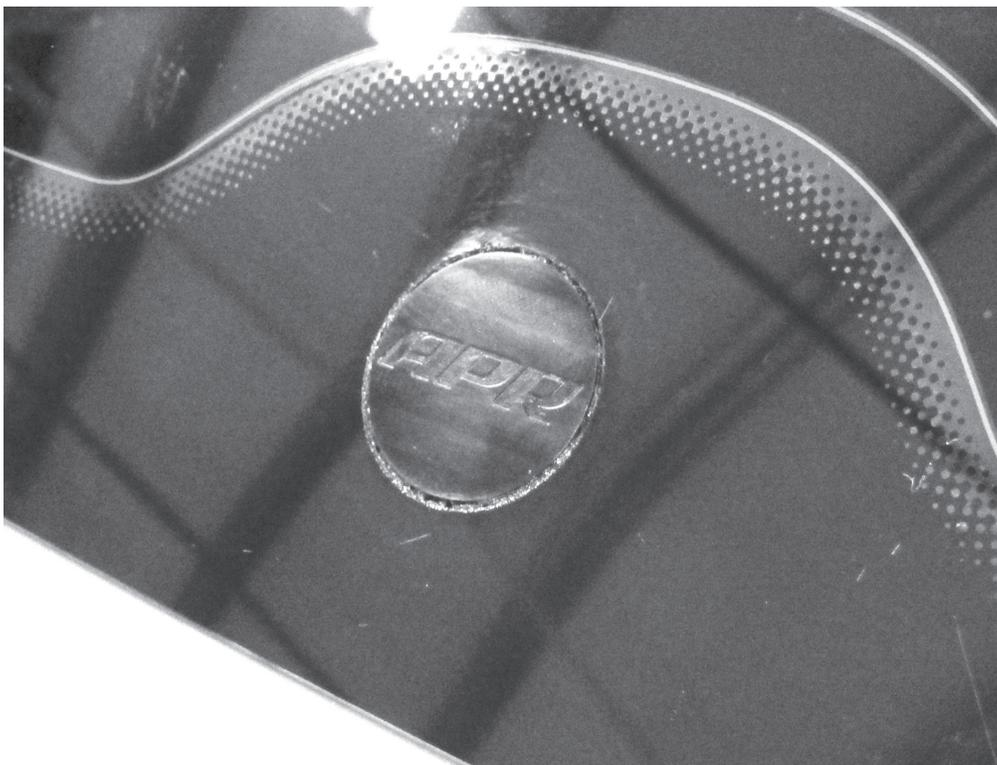
11) Wipe off any excess silicone from the outside of the glass, then allow the silicone to dry. If the vehicle needs to be driven before the silicone cures, apply some masking tape to hold it in place from inside the car.
