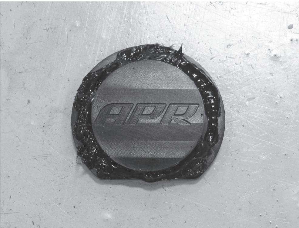
9) Clean the APR wiper delete with an alcohol based cleaner, and then apply the gasket material in a small bead around the wiper delete as shown.
