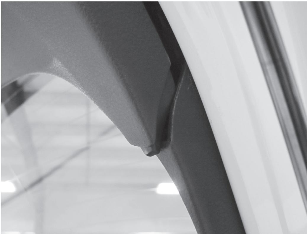
5) Note how the trim panel interfaces with the upper trim panel that surrounds the hatch glass. Remove the hatch trim panel from the car.
