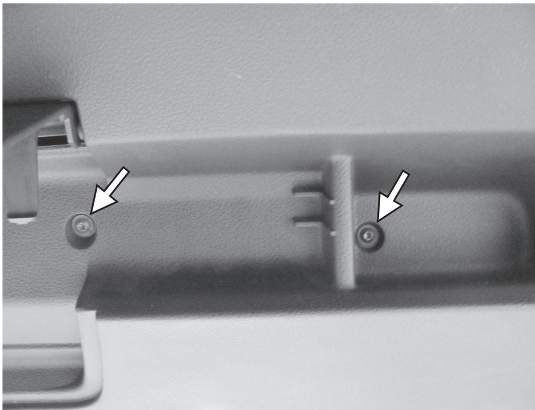
13) Reinstall the screws holding the rear hatch trim panel to the hatch of the car. Reinstall any plastic covers that were previously removed.
