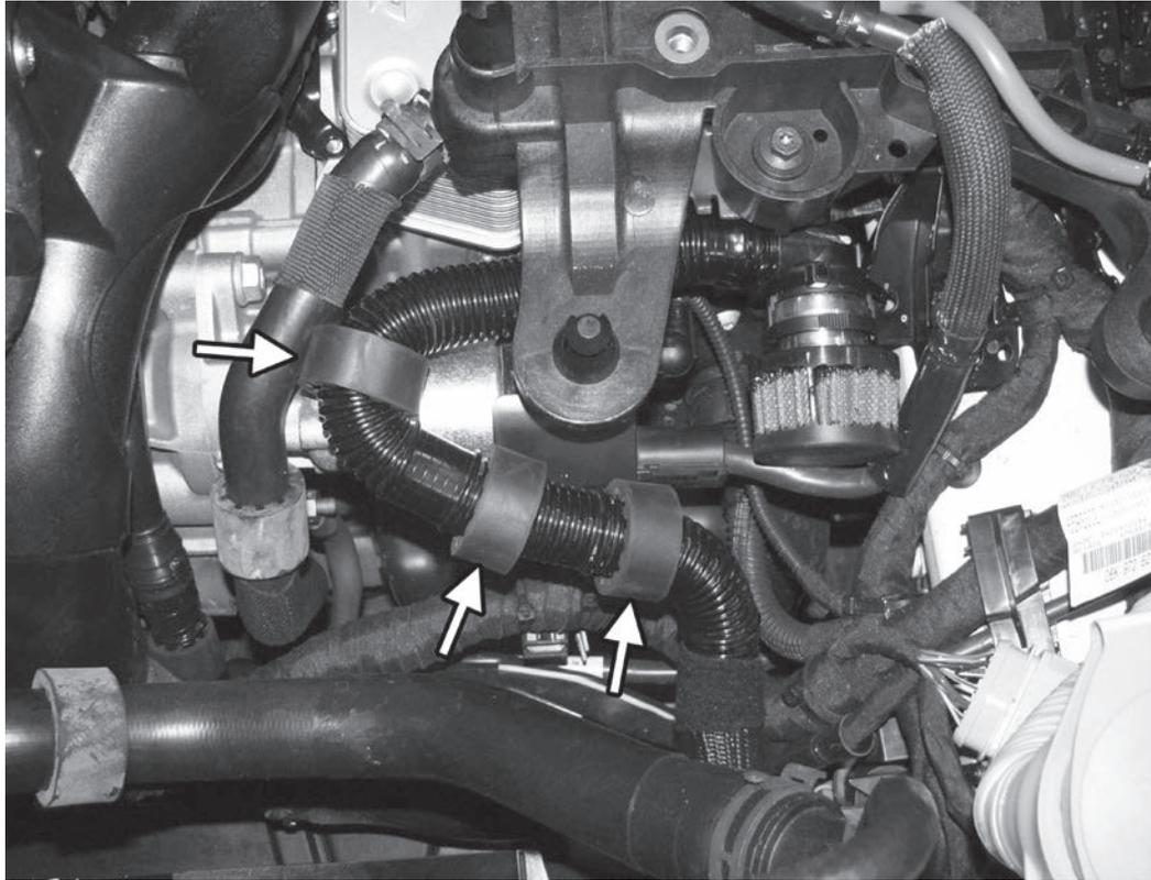
11) If equipped, adjust the three factory rubber bumpers on the secondary air pipe to keep the pipe from rubbing on the engine starter.
