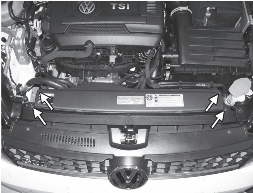
1) Remove the four T25 screws that hold the top cover of the factory air scoop.
