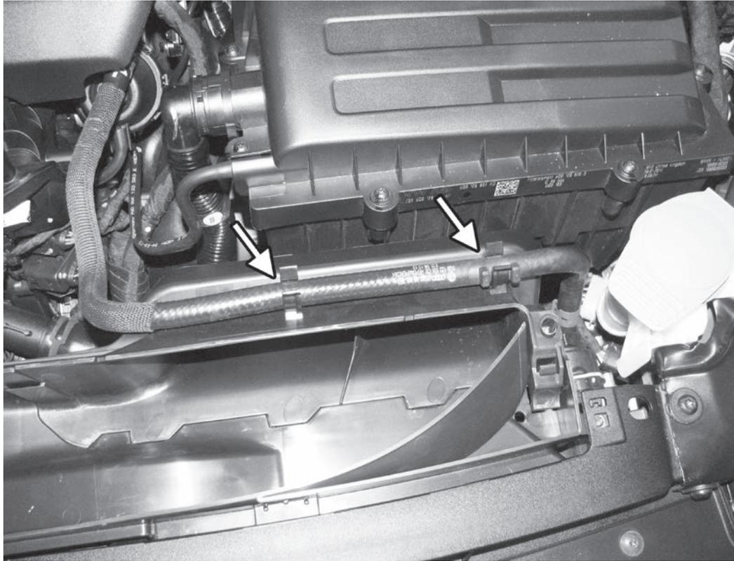
3) Carefully unclip the heater hose from the two tabs on top of the air scoop.
