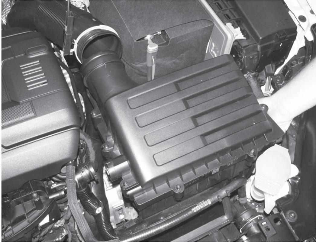
9) Carefully but forcefully lift up on all sides of the factory airbox. The airbox is mounted on three rubber posts underneath, and these must be popped off to remove the airbox from the car.
