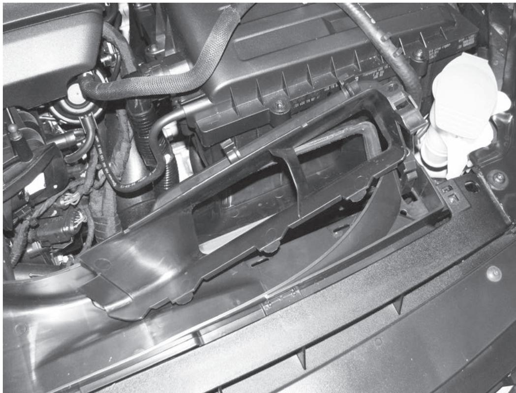
5) Lift the connection to the airbox inlet and remove this piece from the car.
