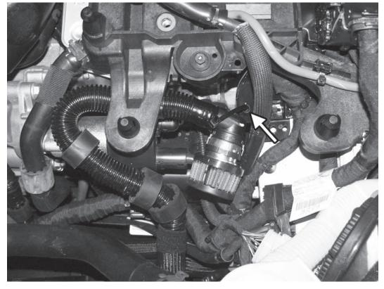
21) If equipped with Secondary Air Injection, clip the APR secondary air filter (Sold separately as CI100020-A) into the factory fitting on the end of the secondary air pipe. Bend the pipe to tuck it out of the way and secure it with the supplied cable ties.
