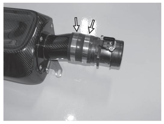
13) Using the supplied silicone coupler and two hose clamps, loosely install the MAF sensor to the back of the APR airbox in the same orientation as the with the stock sensor.
