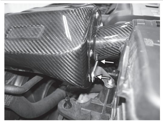
19) Tighten the two 3mm allen screws holding the rear APR bracket to the intake.
