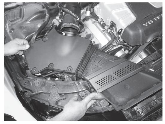
5) Lift the entire airbox assembly with the inlet scoop straight up and remove it from the car. The airbox is attached by two rubber mounting points underneath it, and a mounting bracket on the inside of the right fender.
