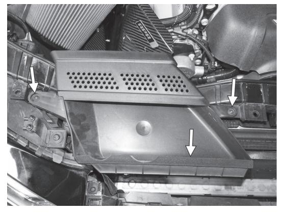
19) Secure the factory inlet scoop to the radiator core support with the two factory T25 screws.
