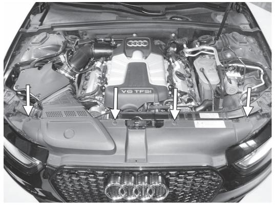
1) Raise the hood of the car. Locate the four pins holding the cover over the radiator. Push the center of each pin in halfway, and then pull the whole pin out and remove all four pins from the cover. Lift the back side of the cover, and pulling towards the back of the car, note how the cover is attached to the top of the bumper. Remove the cover from the car.
