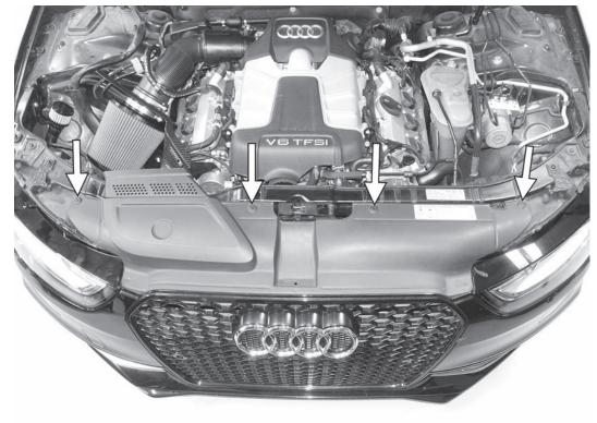
21) Reinstall the cover over the radiator, making sure the front of the cover connects back correctly to the top of the bumper cover. Install the four reset pins in the holes of the upper radiator cover, and then push down on the center portion of the pin to lock the cover in place.
