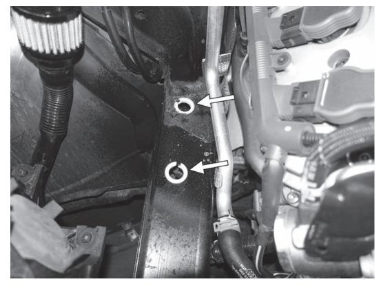
11) Lubricate the mounting holes on the frame rail that the two rubber mounting posts on the bottom of the intake sit in.
