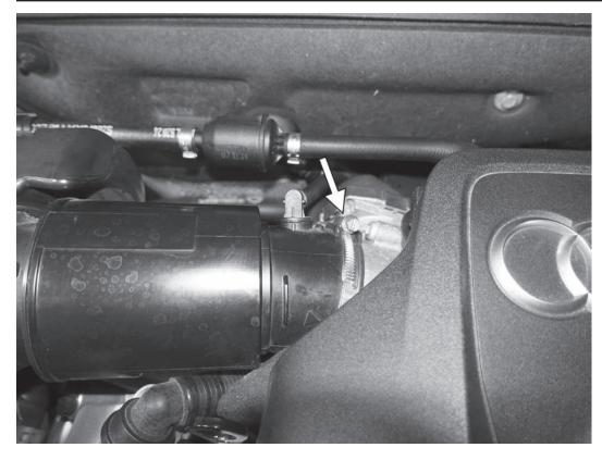
9) Loosen the hose clamp on the back side of the accordian intake tube at the throttle body, but do not remove the tube.
