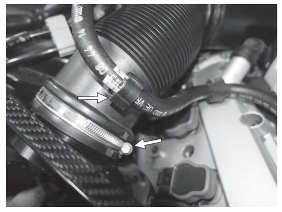
13) Tighten the hose clamp to secure the accordian tube to the APR intake. Also tighten the hose clamp on the accordian tube at the throttle body. Reattach the rubber hose to the clip on the accordian tube.
