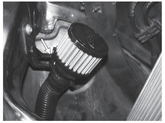
15) Secure the small filter on the end of the secondary air hose with the supplied cable ties to the factory airbox mounting bracket on the inside of the right frame rail.
