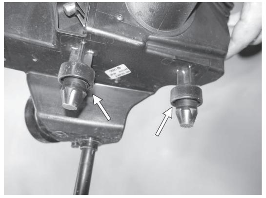
7) From the bottom of the factory airbox, remove the two rubber mounting posts. Note that these posts may have remained in the holes in the frame rail that the airbox sits in and they will need to be pulled out of the frame rail.
