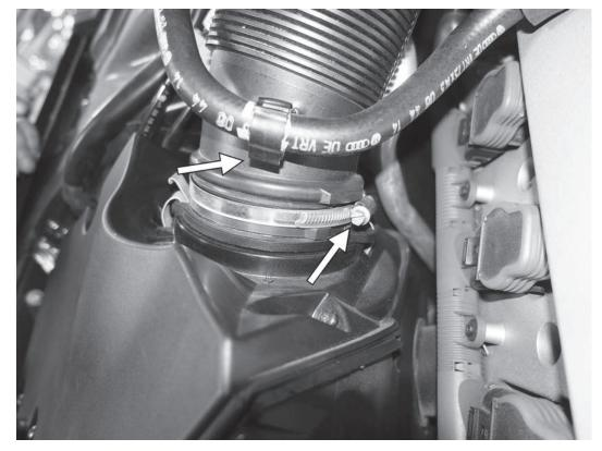
3) Loosen the large clamp connecting the accordian tube to the airbox. Unclip the hose from the side of the accordian tube and detach the hose from the tube.
