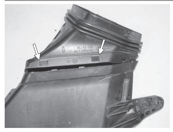
17) Separate the rubber intake tube from the inlet scoop that is secured to the radiator core support by pushing down on all the tabs.
