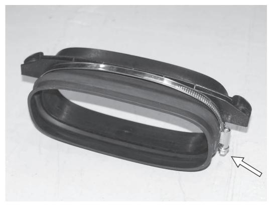
13) Make the shown assembly with the APR airbox adapter, the large supplied coupler, and one of the large hose clamps. Note the orientation and positioning of the hose clamp relative to the APR adapter.
