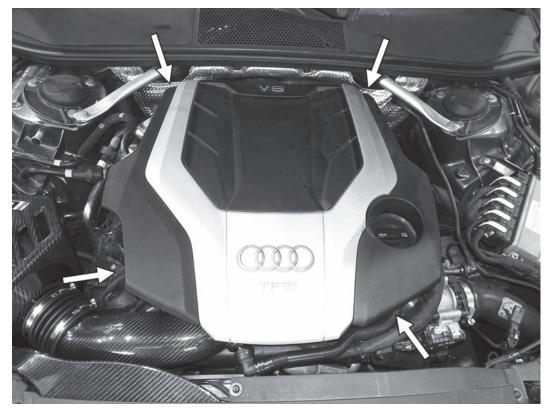
31) Reinstall the engine cover by pressing the cover down onto the four mounting posts on the engine.
