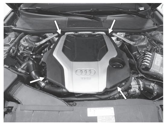
1) Raise the hood and remove the engine cover by lifting on each of the four corners of the cover.
