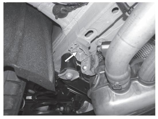
7) Remove the two 13mm bolts holding both rear exhaust hangers to the muffler section.
