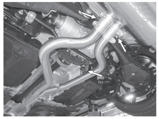
19) Loosely install the rear section assembly with two of the supplied APR sleeve clamps to the rear muffler as shown. Connect the exhaust mounting post onto the factory rubber hanger on the right side.
