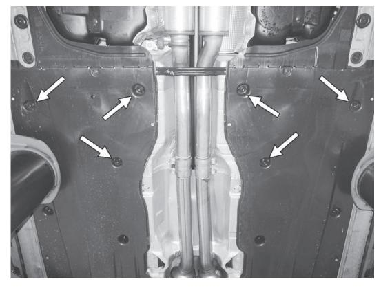
1) Support the car on a lift or jackstands. Remove the six 10mm from the rear fasteners on both side underbody panels.
