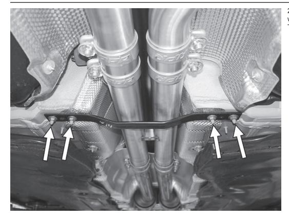
23) Reinstall the factory crossbrace with the four original 13mm nuts. Tighten the nuts to 20Nm (15 ft-lbs).
