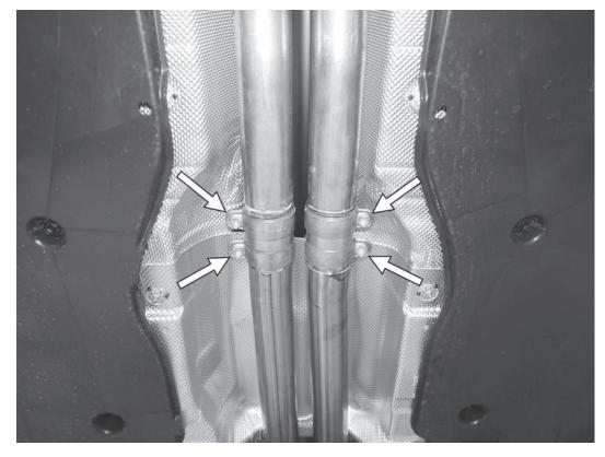
3) Loosen the 13mm nuts on the two exhaust clamps at the center of the exhaust, but do not slide the clamps out of their current location.
