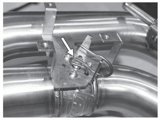
13) If your exhaust valve configuation had the D-shaped spring instead of the spiral spring, install the D-shaped spring onto the slot on the top of the APR valve. The arm of the spring should be mounted fully clockwise between the two "stop" posts on the bracket.
