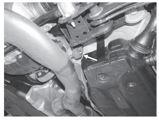
5) Disconnect the two rubber hangers from the center of the exhaust system (the one shown and the one slightly further forward on the left side), leaving the hangers attached to the car.
