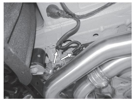
17) Reconnect the wiring harness to both exhaust valves, and then reattach the harness clips onto the metal exhaust hanger bracket.
