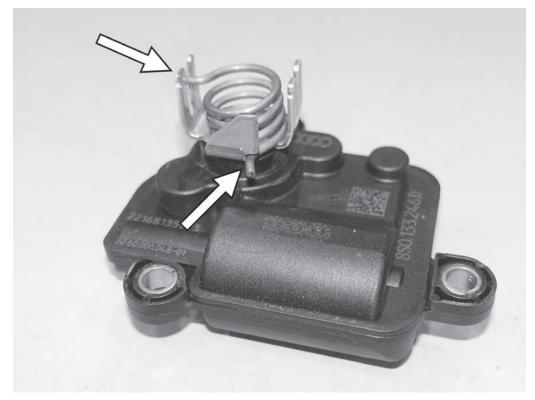
11) Install the factory spring on the factory exhaust valve motor as shown. One tab of the spring connects to the notch near the base of the valve motor, and one tab goes between two of the vertical tabs on the motor.
