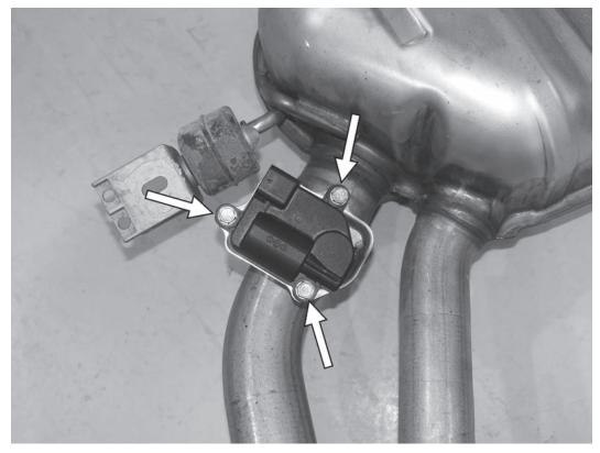
9) Remove the six 10mm screws holding both exhaust valve motors to the rear muffler assembly, and remove the valve motors from the exhaust. Also remove the springs that were between the valve motors and the valve.
