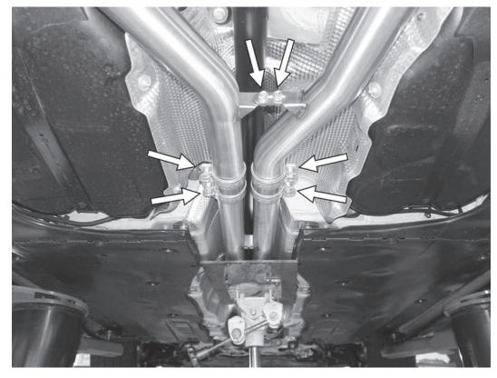
21) Support the front section of the exhaust, making sure it sits correctly in the center exhaust tunnel. Tighten the 13mm nuts on the factory sleeve clamps to 23Nm (17 ft-lbs). Tighten the 15mm nuts on the APR sleeve clamps to 35Nm (26 ft-lbs). Then, tighten the 13mm screws on the cross brace on the APR rear section to 10Nm (88 in-lbs).
