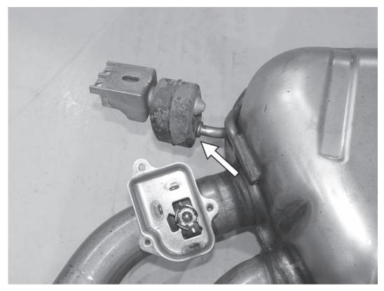
15) Remove the two exhaust hanger brackets with rubber mounts from the factory exhaust, and install them onto the APR exhaust in the same locations.
