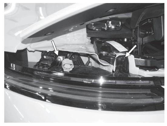
57) Secure both rear side taillights with the four T30 screws. Remember the spacer on the two outer screws. Tighten all four screws to 6Nm (53 in-lbs).
