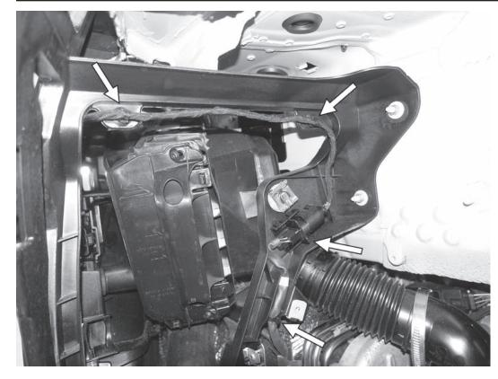
19) Separate the electrical connector for the oxygen sensor from the airbox frame, and then unplug the electrical connector. Then separate the clips on the harness from the airbox frame. Repeat this on the other side of the car.
