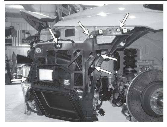
23) Remove the five 10mm nuts and one 10mm screw holding the airbox frame to the car. Repeat on the other side of the car.
