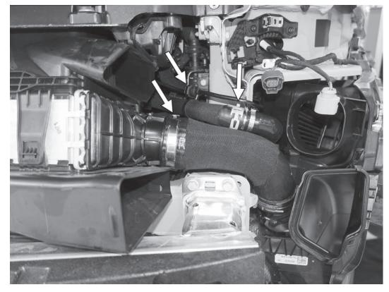
41) Reconnect the intercooler inlet hose to the intercooler and secure the stock clamp to 5.5Nm (49 in-lbs). Reconnect the vacuum line to the airbox at the factory coupler. Reconnect the diverter valve line to the APR coupler on the APR diverter valve hose and secure with the factory spring clamp. Repeat on the other side of the car.
