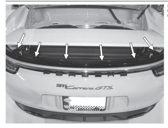
59) Secure the center taillight with the six T30 screws, and then tighten the screws to 6Nm (53 in-lbs).
