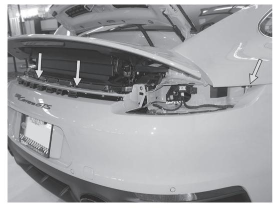
55) Reinstall the two remaining T30 screws to the top of the bumper cover. Tighten all two rear T30 screws to 3.2Nm (28in-lbs). Tighten the two previously installed outer T30 screws to 7Nm to (62 in-lbs).
