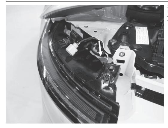
39) Reinstall both rear side taillights. Reconnect the electrical connectors on the lights before pushing them forward into their mounting locations.
