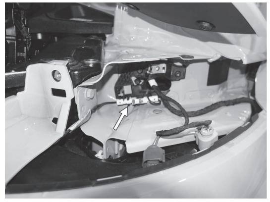
33) Reconnect the electrical connector from the right side of the rear bumper wiring harness to the area where the right taillight was. Some cars may have more or less electrical connectors depending on the vehicle options.
