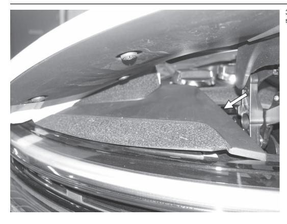
3) Pop out the plastic panels on both sides of the rear decklid spoiler.
