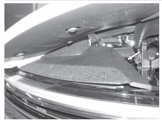
43) Snap back in the plastic panels on both sides of the rear decklid spoiler.
