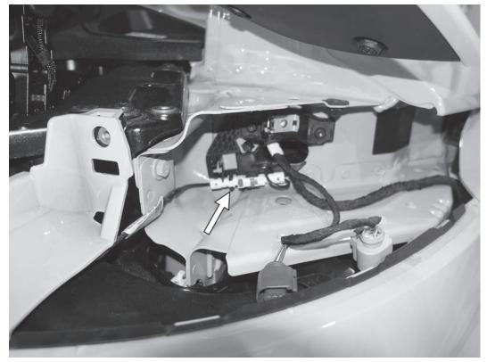
13) Disconnect the right side of the rear bumper wiring harness from where the right taillight was. Some cars may have more or less electrical connectors depending on the vehicle options.
