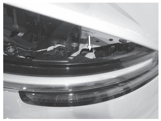
41) Place the center taillight back onto the car, and then reconnect the electrical connectors on both sides of the light. Push the taillight forward into its mounting location.
