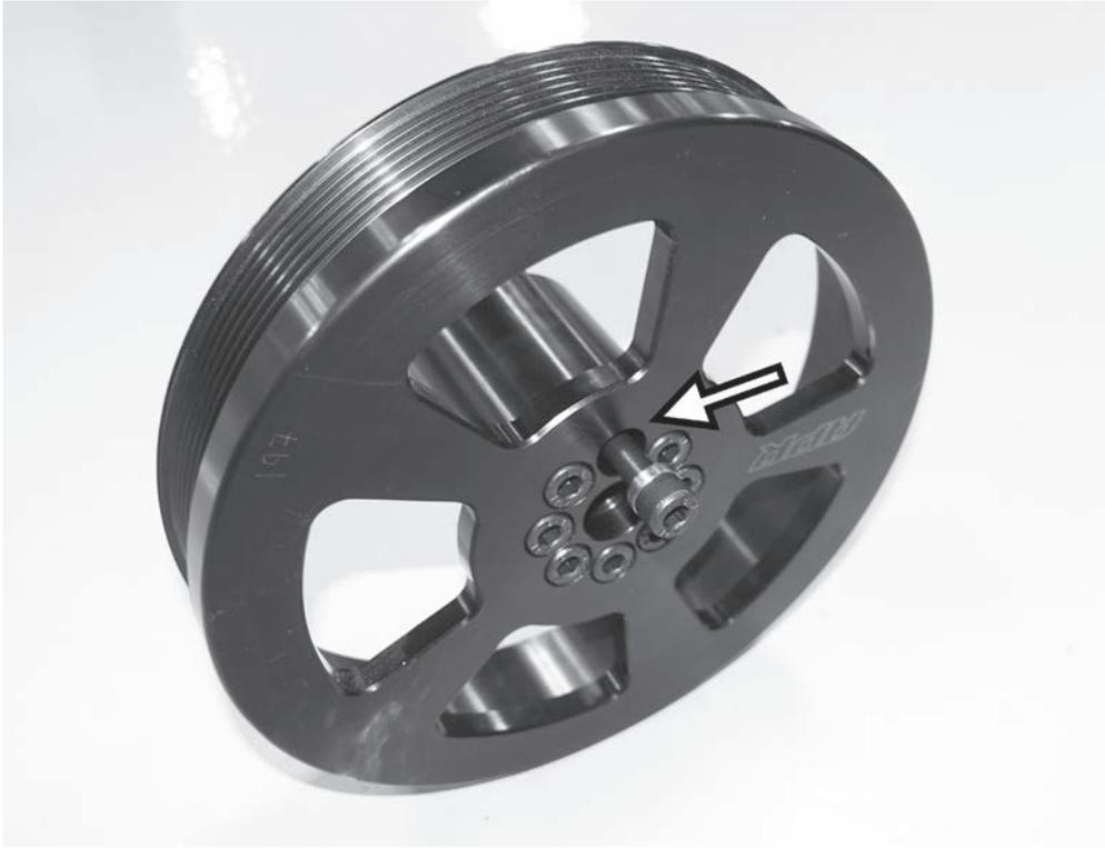
21) Install the 8x supplied bolts with washers into the APR crank pulley. Note that one of the holes on the APR pulley is slightly offset from the others.
