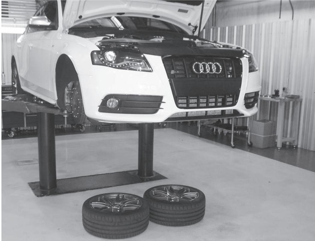
1) Securely lift vehicle. If a vehicle lift is not used, secure the vehicle with jack stands. Remove both front wheels.
