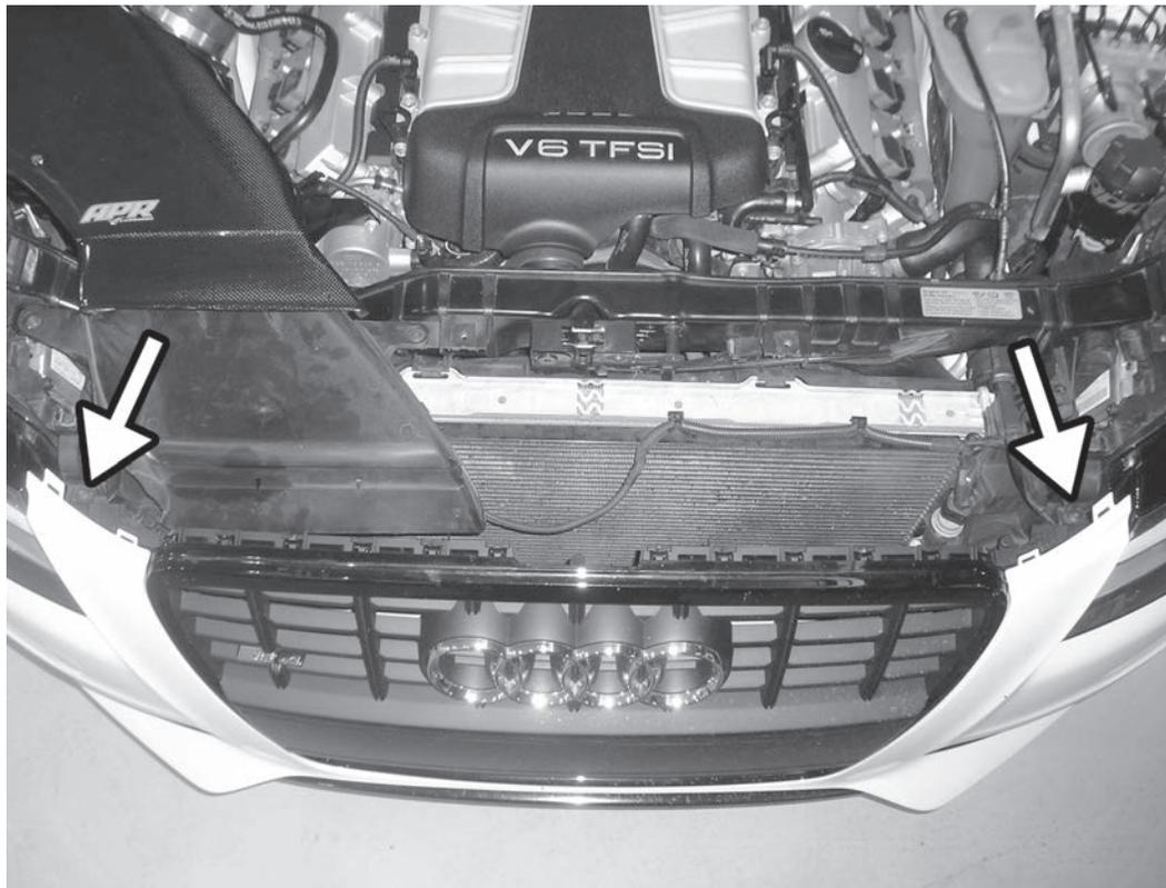
7) Remove 2x T25 Torx screws from top of bumper cover.
