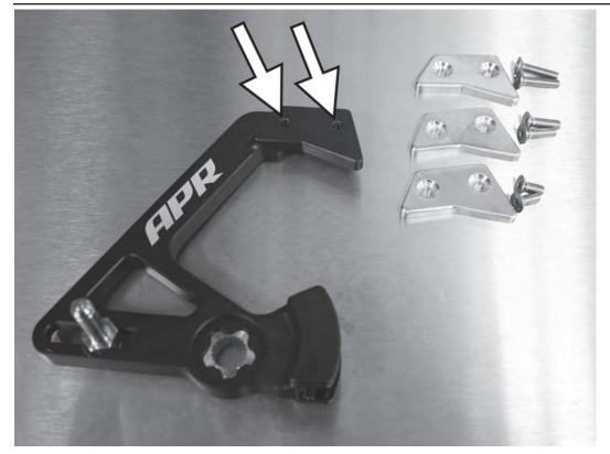
15) Select the amount of inertia weight you wish to use. Select the appropriate length screws for the number of weights used. When installed, the screws should not protrude from the bottom of the primary lever. Install the weights to the primary lever, and tighten the 4mm allen screws to 2Nm (18in-lb).
