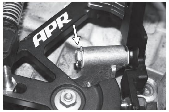
19) Grease and install the other relay lever bushing into the other side of the mounting hole. Attach the supplied retaining clip to the pivot pin, locking the relay lever to the transmission.
