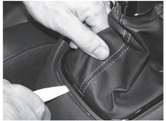
21) Inside the car, gently lift up on the boot around the shifter, and then using a plastic trim tool, carefully pry the shifter surround trim up. There are two locking tabs on the back of the shifter trim.
