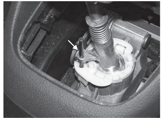
31) Remove the locking pin from the shifter inside the car. Replace the sound deadening absorber and reinstall the shifter surround trim by pushing the securing clips back in place. Make sure the shifter freely goes into each gear, including reverse.
