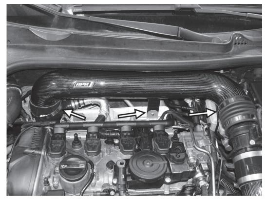
11) Place the supplied hose clamp on the top of the APR inlet coupler. Set the APR intake pipe in place, sliding the support bracket between the washer of the T30 screw and the metal tab on the heat shield. Slide the intake pipe into the inlet coupler, and put the accordian coupler onto the back of the MAF housing.
