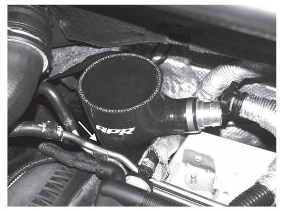
7) Place the APR inlet coupler all the way down onto the turbo inlet. Then rotate the coupler so the PCV hose will easily connect to the port on the side of the APR inlet coupler. Secure the coupler with the spring clamp.
