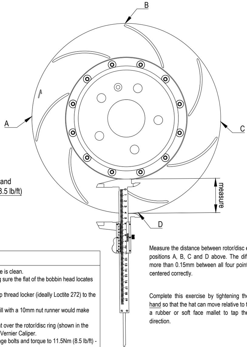
Measure the distance between rotor/disc edge and hat flange at positions A, B, C and D above. The difference should be no more than 0.15mm between all four points to ensure the hat is centered correctly.
