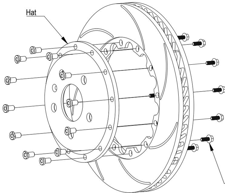
Apply thread-locker and torque to 11.5Nm (8.5 lb/ft)
