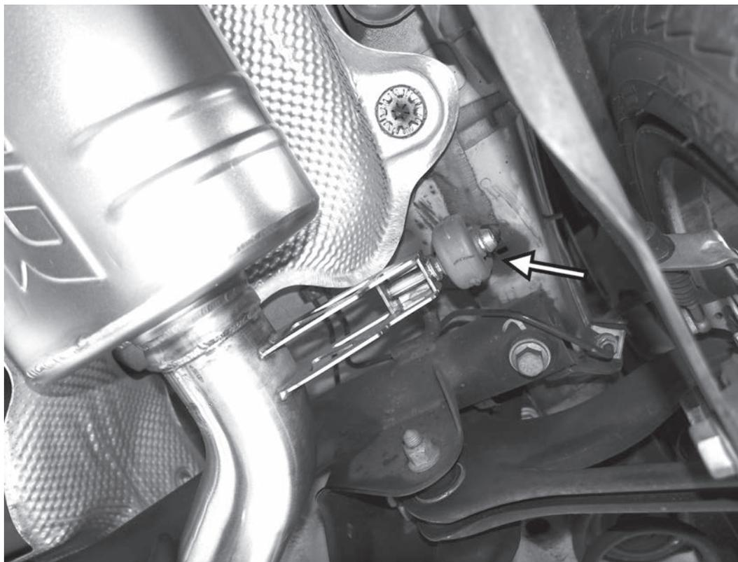
13) With an assistant, lift the APR muffler section to the car, and attached the rear hanger of the muffler section to the previously installed rubber hanger near the rear axle.
