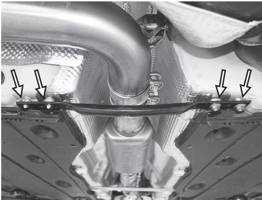
25) Reinstall the rear brace with the four supplied spacers between the brace and the chassis of the car. Use the original 13mm nuts to hold the brace with the spacers in place.
