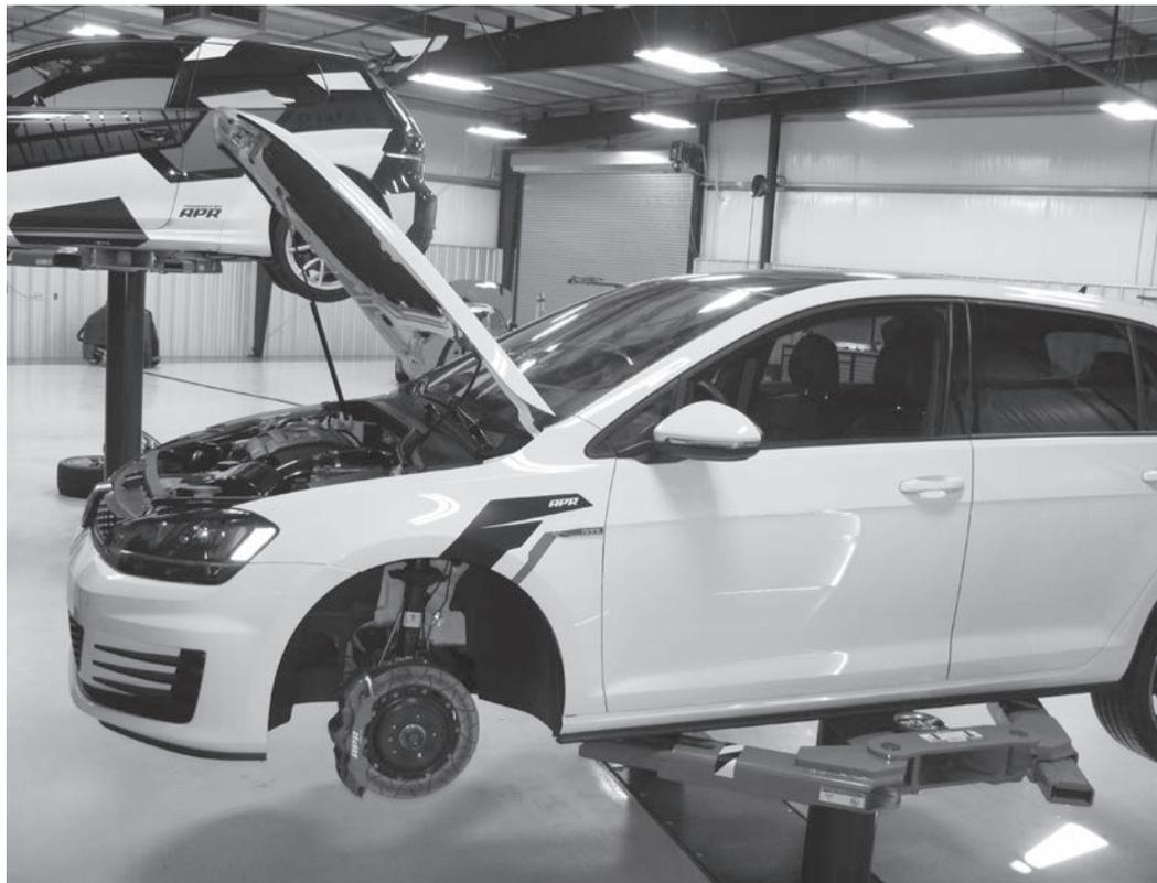
1) Securely lift vehicle. If a vehicle lift is not used, secure the vehicle with jack stands. It is not necessary to remove the wheels, but will make installation easier.
