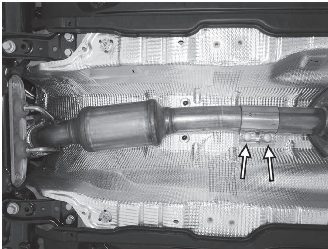
3) If the car has a stock DP, loosen the two 13mm nuts on the stock sleeve clamp at the back of the DP.
