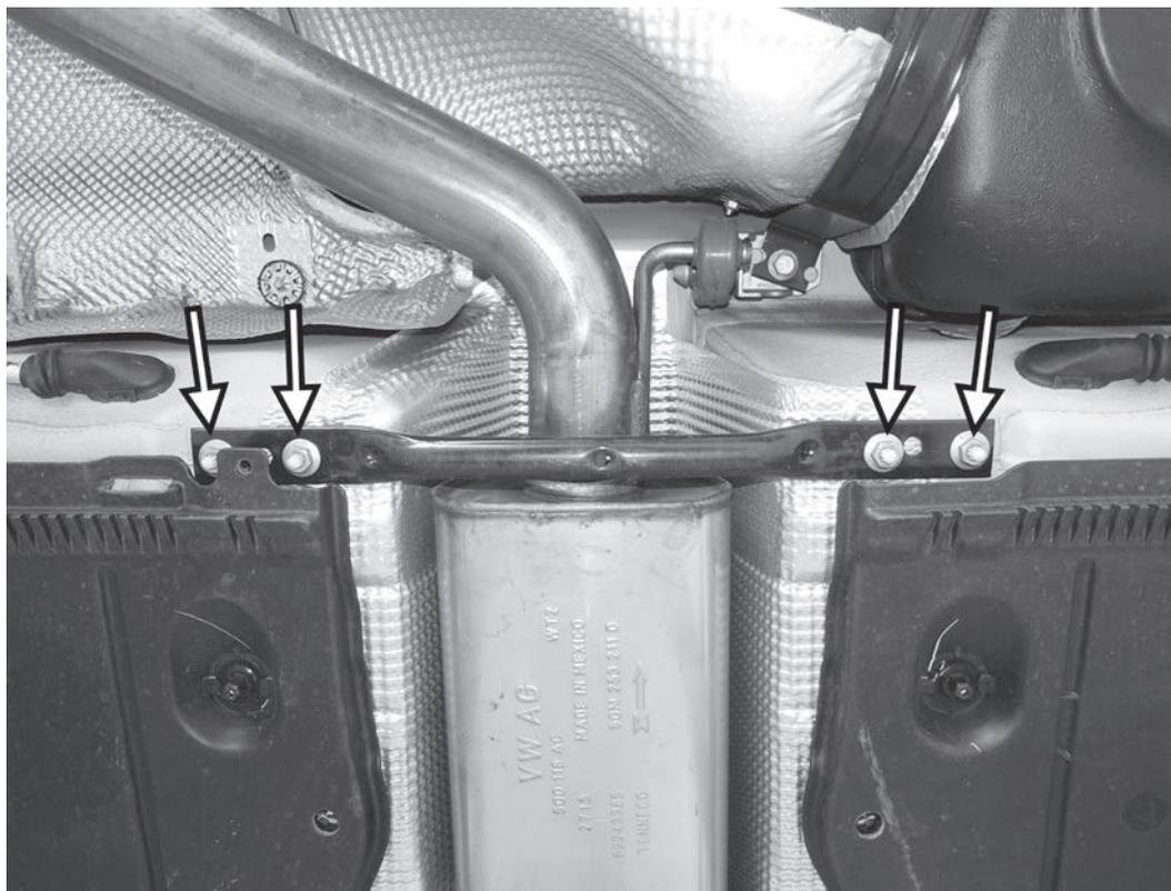
5) Remove the four 13mm nuts holding the brace at the back of the center tunnel, and remove the brace from the car.
