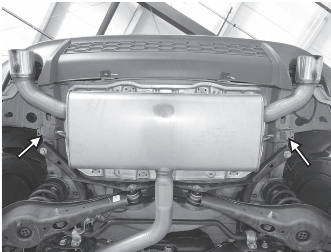
7) With an assistant holding the exhaust so it does not fall, remove the two 13mm bolts holding the rear muffler hanger brackets to the car.
