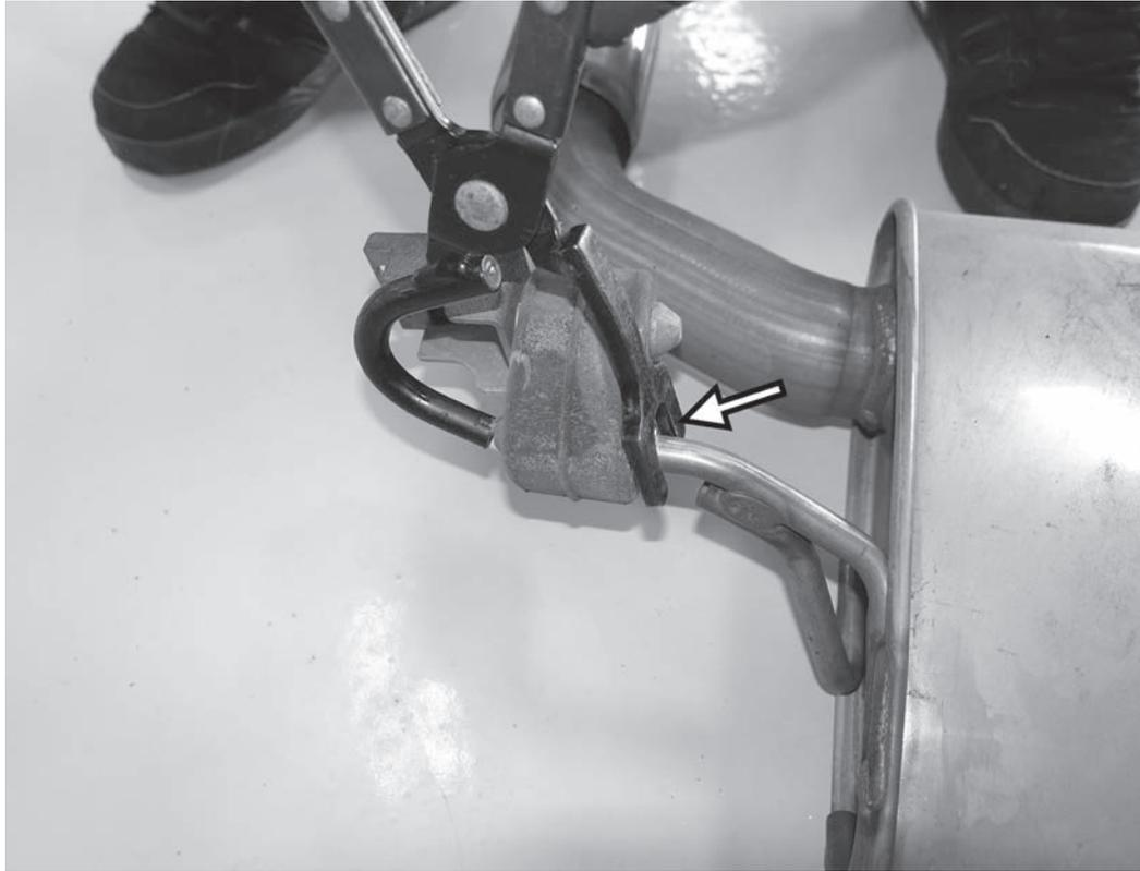
17) Put some spray lubricant on the rubber hangers on both sides of the stock rear muffler. Remove the two hangers with attached brackets from the exhaust. The hangers can be separated from the exhaust with a pry bar or a tool made to remove rubber hangers.
