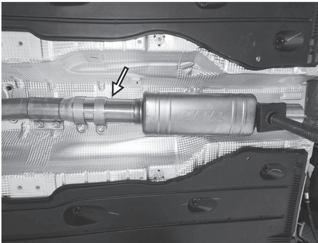
11) Loosely place the APR resonator or straight pipe into the back of the previously installed APR sleeve clamp. If installing the resonator, it should be oriented so the APR logo is facing the same direction as the APR logo on the muffler that is about to be installed.
