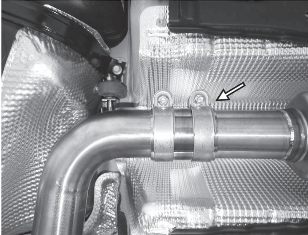
15) After confirming the orientation of the resonator is correct (the APR logo is in the same direction as on the muffler), slide a sleeve clamp on between the two sections. Loosely tighten the sleeve clamp so it can still be manipulated.
