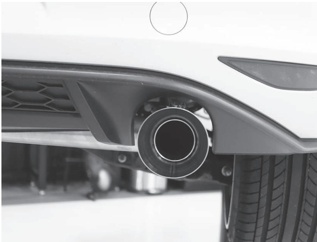
23) Adjust the exhaust tips to your desired position before tightening the pinch clamps to 55Nm (40 lb-ft). Verify tip is securely in place.
