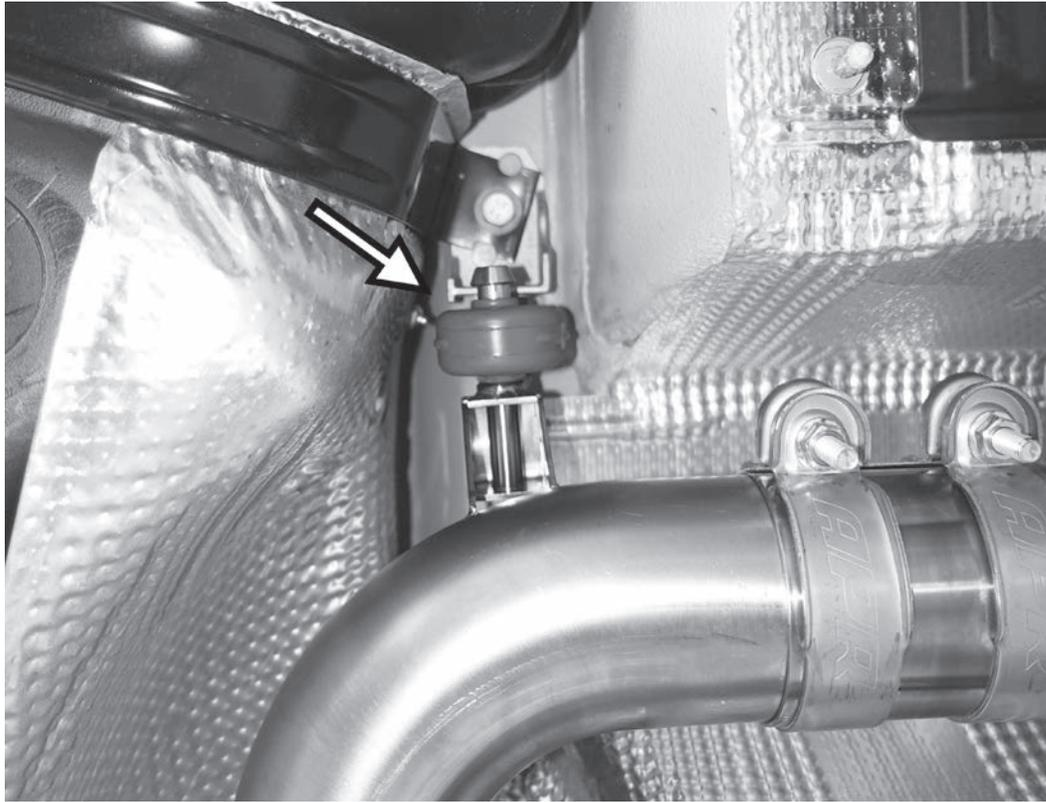
21) Working from the front of the car to the back, adjust the APR exhaust so all rubber hangers are facing straight down. The posts of the APR exhaust should hang directly below the factory posts the rubber hangers sit on. Once aligned, torque the sleeve clamps in the center tunnel of the car beginning with the most forward one to 25Nm (18 lb-ft).
