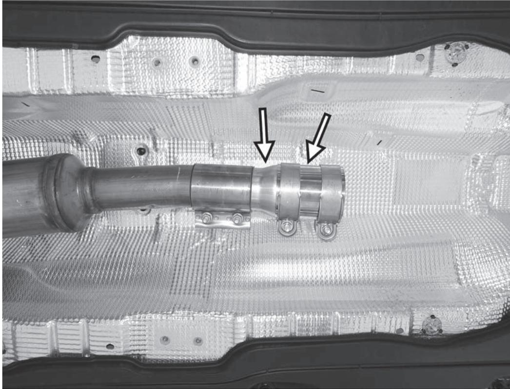
9) If installing with a stock DP, loosely place the small end of the reducing coupler into the stock sleeve clamp on the end of the stock DP. Loosely install one of the APR sleeve clamps on the big end of the reducing coupler.
