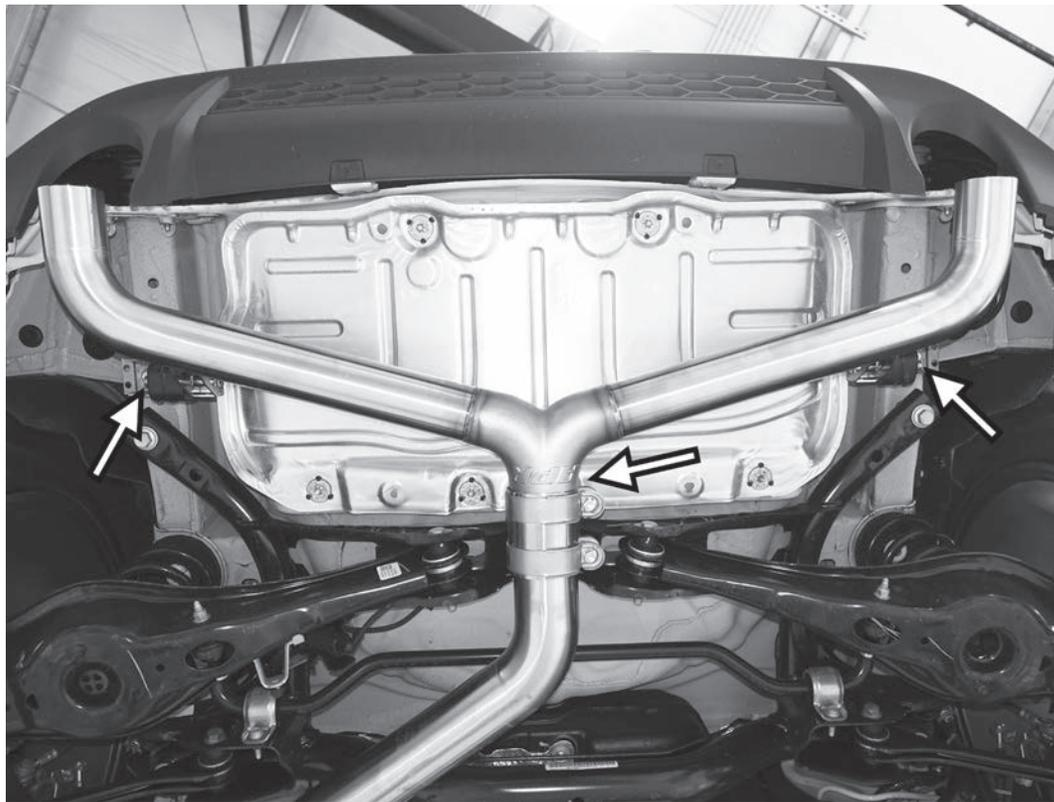
19) Slide the front portion of the APV rear section into the sleeve clamp on the back of the APV muffler section. Loosely install the two original 13mm bolts on either side of the back of the car, reattaching the rubber hanger brackets back to the car.
