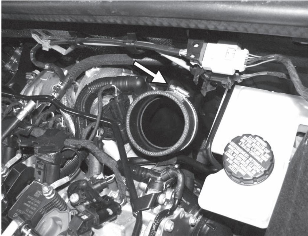
3) Install the straight APR silicone inlet coupler to the factory turbo inlet pipe and secure with one of the supplied 8mm hose clamps.
