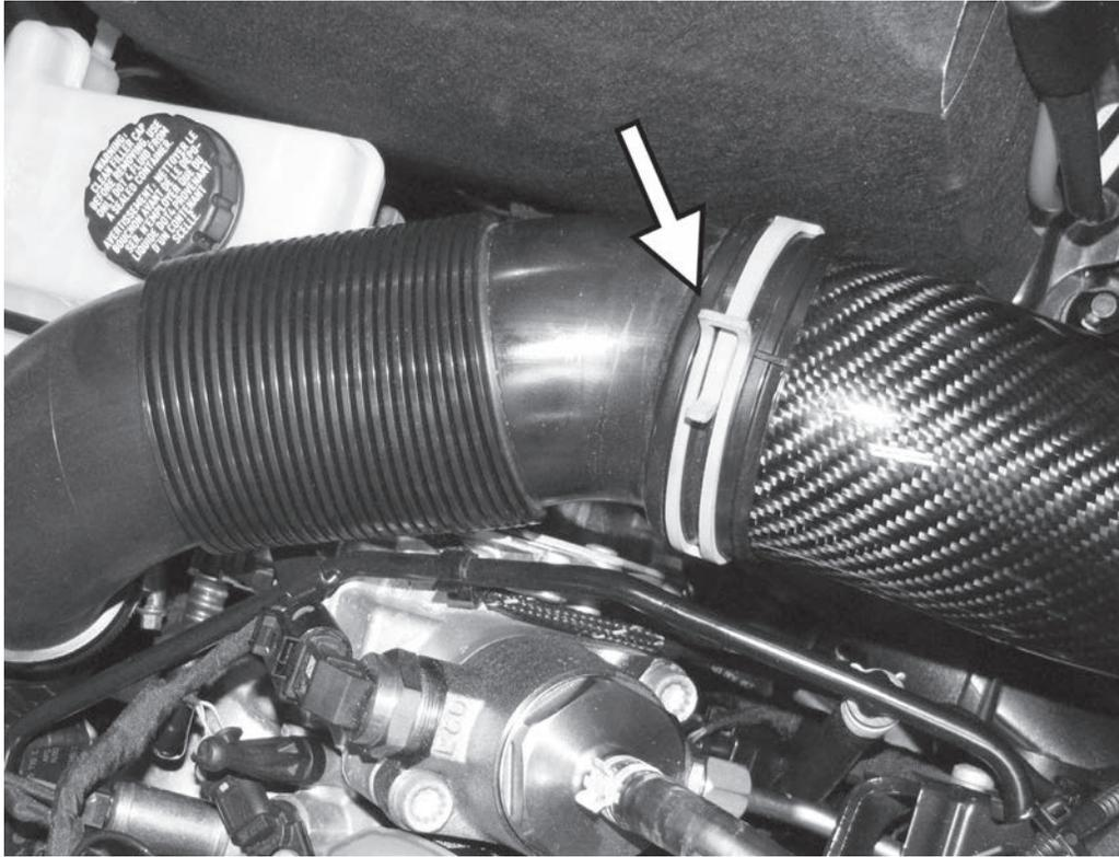
1) Remove the factory engine cover by lifting up on the corners of the cover and lifting up. Remove the spring clamp holding the back of the APR intake to the factory accordion inlet tube by sliding the clamp over the inlet tube.
