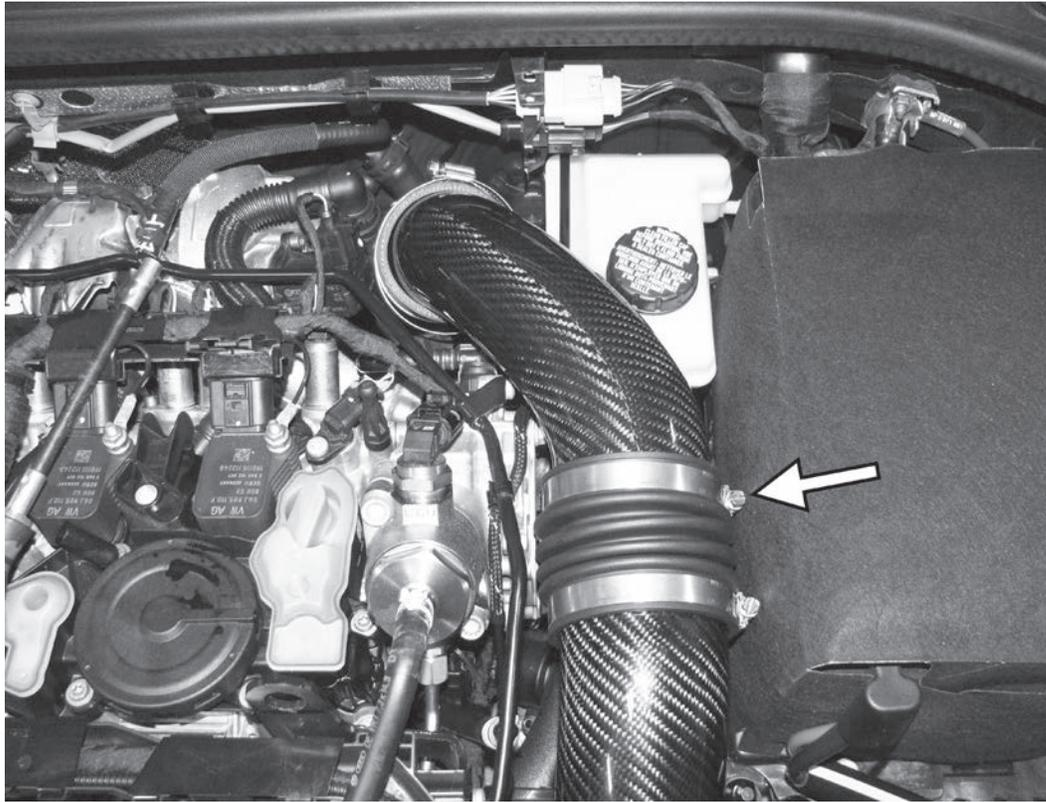
5) Install the APR Stage 2 pipe between the two couplers. Secure the front side of the pipe to the APR accordion coupler with one of the supplied 8mm hose clamps.
