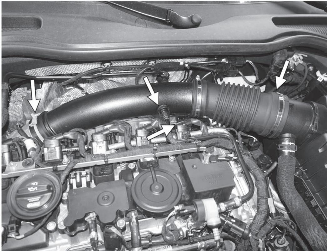
57) Install the stock intake tube between the accordian hose and the airbox. Install the T30 screw holding the tube to the cylinder head and torque to 80 in-lb (9Nm). Reconnect the Norma style fitting from the crankcase solenoid valve (N546). Install the spring clamp from the intake to the stock compressor inlet pipe. Finally, install the screw clamp holding the intake to the airbox and torque the clamp to 48 in-lbs (5.5Nm). Reinstall the engine cover.
