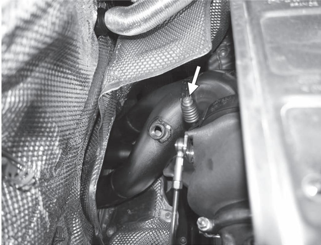
53) Fully secure the V-Band clamp on the downpipe by torquing the T25 screw to 62 in-lb (7Nm).
