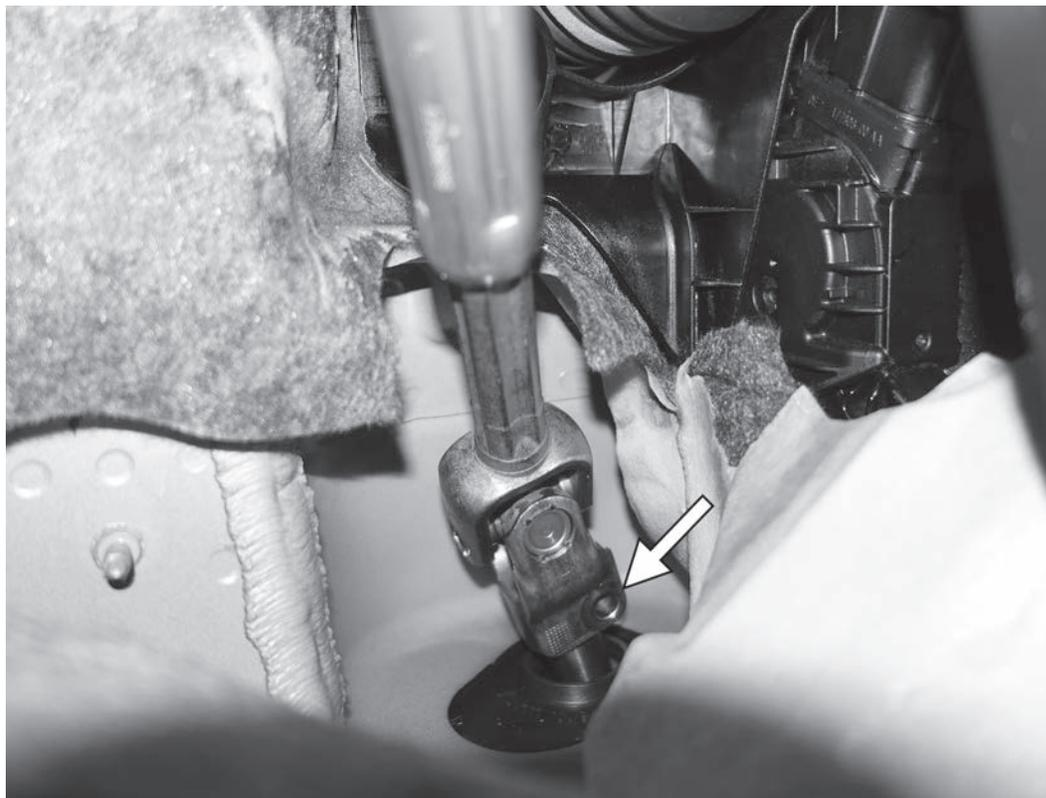
3) After making sure the steering wheel is centered, fold down the carpet, and remove the 13mm bolt holding the steering column to the steering shaft. Lift up on the steering column to separate it from the steering shaft.
