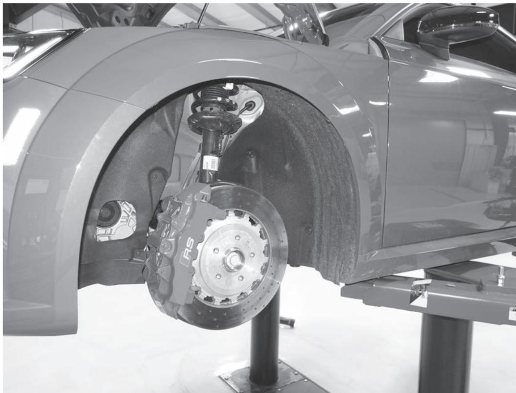
1) Securely lift the car using an auto lift or a jack and jackstands, then remove the front wheels.
