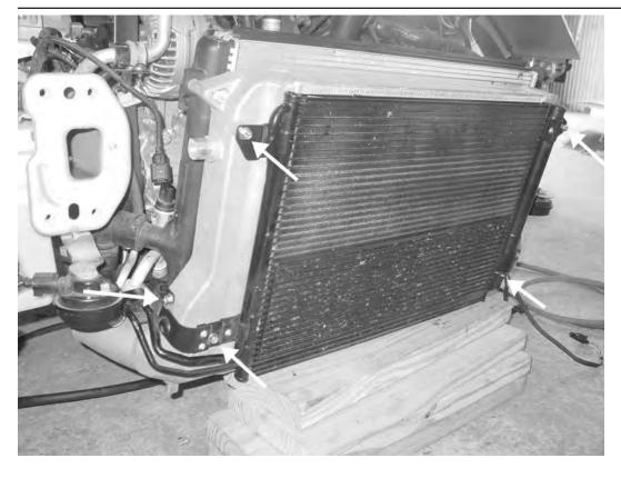
29) Connect the condenser to the APR intercooler using the five 10mm bolts. These five bolts connect the condenser to the APR intercooler in the same locations as the stock intercooler. Be sure to install the side condenser hose bolt first before trying to install the four bolts on the front of the condenser.
