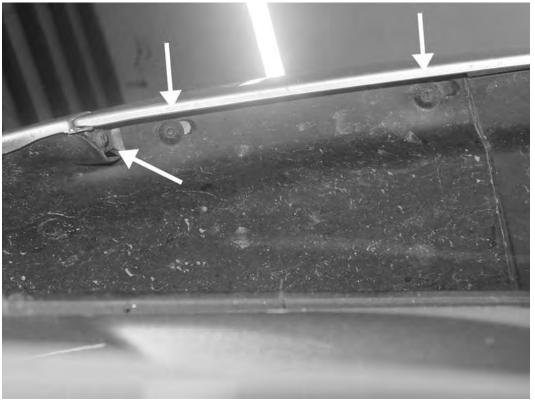
51) Reinstall all of the T25 Torx screws that connect the bumper to the wheel well liners, including the two T25 Torx screws that connect the bumper to the fenders.
