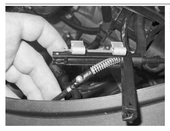
47) Reconnect the hood release cable and reconnect the housing with the factory clips behind the drives side headlight. Confirm that the hood release works from inside the car before closing the hood.
