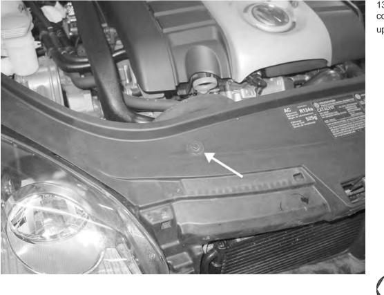
13) Remove the 8mm bolt that connects the noise booster to the upper radiator support.
