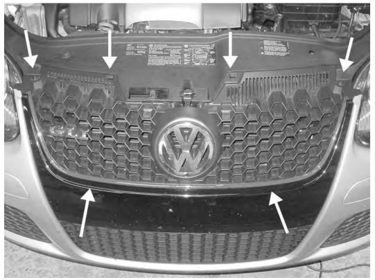
53) Place the bottom of the radiator grill into its original location, and install the two Phillips screws. Rotate the top of the radiator grill back, snapping the two upper center clips into place. Reinstall the two T25 upper screws on the radiator grill.
