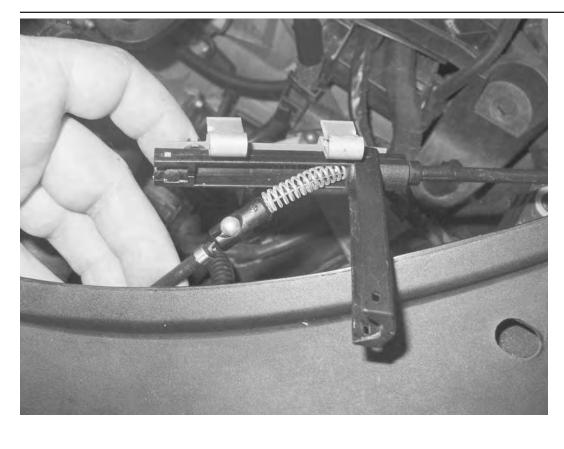
11) Unclip the hood release coupling located above the driver's side headlight. Open the coupling with a small screwdriver and release the cable.
