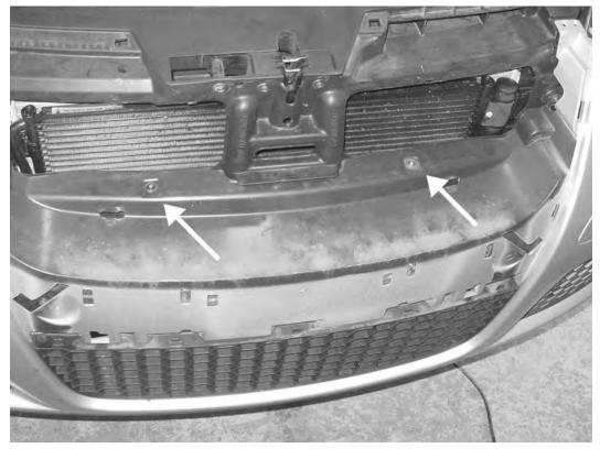
7) Remove the two T25 Torx Screws and the two T30 Torx Screws on the top of the bumper that were revealed when the radiator grill was removed.
