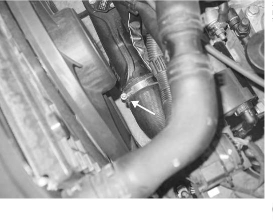
21) Loosen the hose clamp on the passenger side intercooler hose from above the car.
