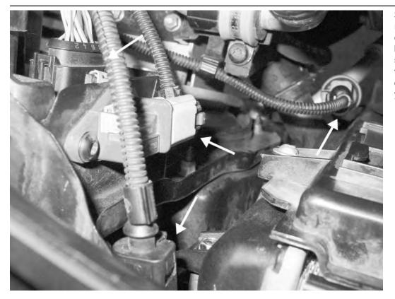
37) From the top of the car, reconnect the following electrical connectors: A/C pressure sensor, both headlights, and the hood latch sensor. Again, after confirming the battery on the car is still disconnected, reconnect both of the yellow airbag crash sensors.
