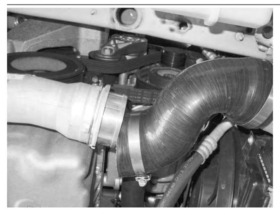
45) Making sure the locking clip is pulled away from the stock coupling on the car, install the APR coupling adaptor. Then install the APR passenger side intercooler hose using the two supplied hose clamps. Connect the two ends of the hose, make sure the hose is oriented without any kinks, and tighten both hose clamps in place.
