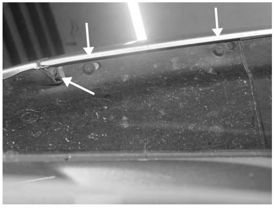
5) Remove the T25 Torx Screws that run along the inside of the front of the wheel wells. These connect the fender liner to the bumper. Also remove the two screws that connect the bumper to the fender.
