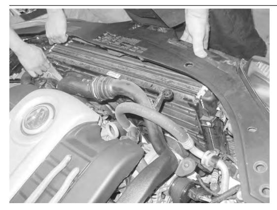
23) With a partner, remove the two APR-supplied bolts from both sides of the radiator core support. Remove the condenser/intercooler/ radiator/fan assembly from the core support by sliding the upper part of the intercooler assembly away from the top of core support. While doing this, the intercooler side grommets will side out of the core support. Once the side grommets of the intercooler are free, lift the intercooler assembly up and out of the core support. Set the core support aside.
