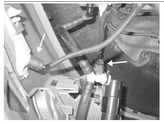
49) Reconnect the foglights and sidemarker electrical connections on both sides of the bumper.
