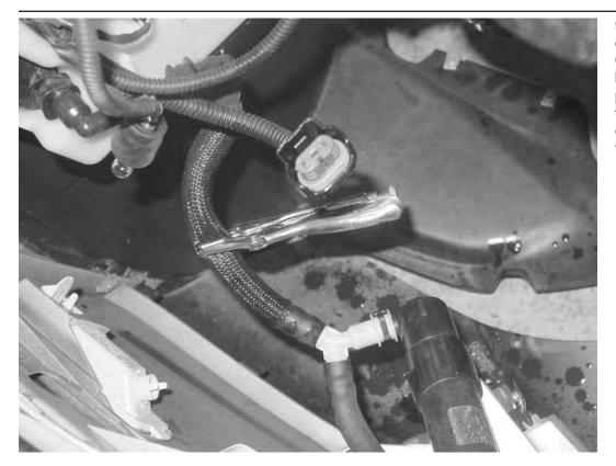
9) With a partner, slide the bumper cover forward several inches. Clamp the headlight washer line before the "T" with a suitable tool to prevent washer fluid loss. Remove the washer lines from the clips at each washer, and separate the line from the clips in the bumper. 10) Remove the bumper and carefully set aside as not to scratch the paint.
