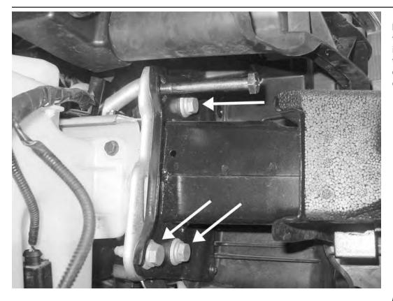
15) Remove the remaining six 16mm bolts from the car and carefully pull the radiator core support forward an inch or two. Be careful not to stretch the two air conditioning lines located on the passenger side of the A/C condenser.
