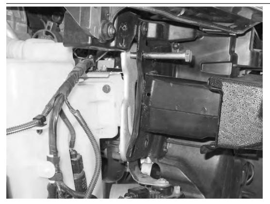
39) Making sure all connectors and hoses are clear, push the radiator core support back to where it is touching the front frame rails.
