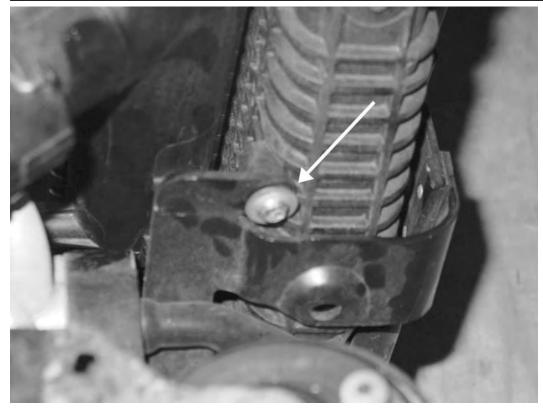
25) Begin to separate the A/C condenser from the intercooler by removing the four T30 screws from the front of the condenser. There is also one T30 screw on the passenger side holding the condenser lines to the intercooler. These five screws are not reused.
