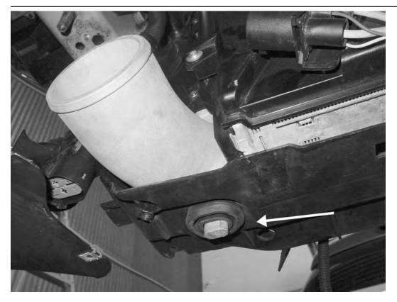
33) From underneath the car, lift up on the intercooler/condenser/ fan assembly and set the bottom "feet" of the APR intercooler into the rubber grommets on the core support. 34) Rotate the top of the intercooler into the core support, making sure the side intercooler grommets mount into their respective locations on the radiator core support.
