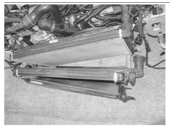
27) Carefully maneuver the stock intercooler out of the car from between the condenser and the radiator.
