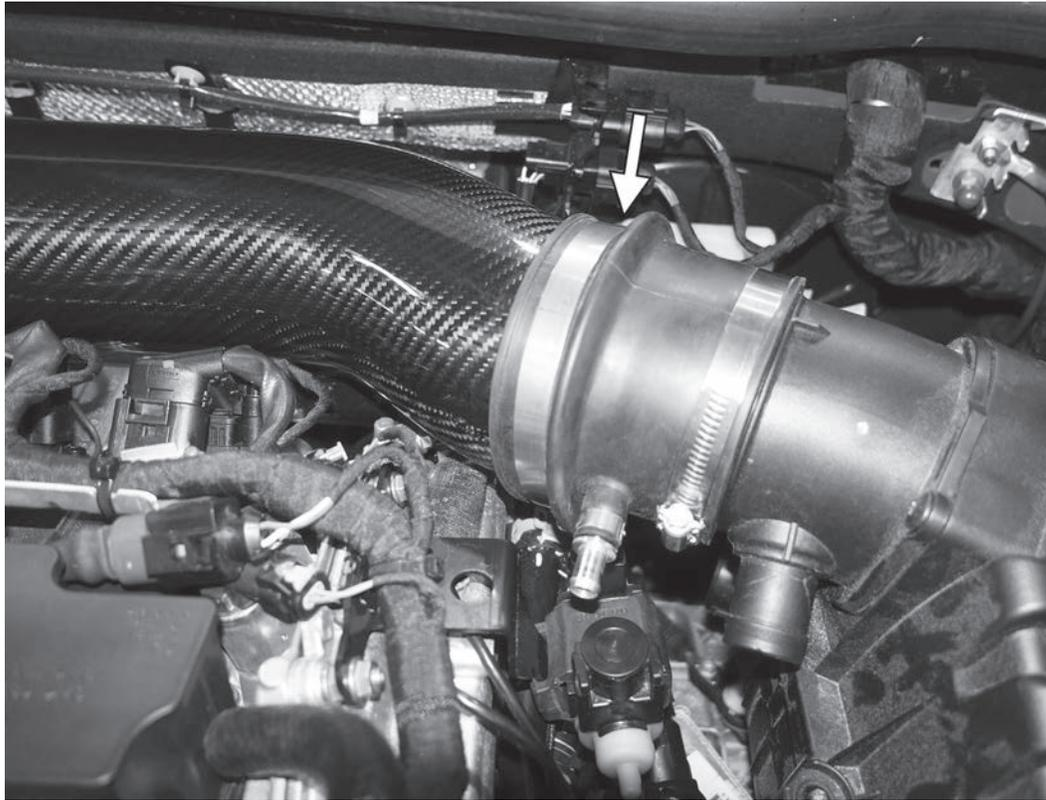
9) Loosen the screw clamp holding the airbox elbow to the APR rear inlet pipe. Lift up on the airbox assembly to separate it from its rubber mounting posts and remove the airbox assembly from the car.
