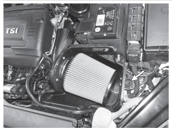
9) Place the APR intake in the car, ensuring the three rubber mounts connect to the three mounting posts the factory airbox was connected to.
