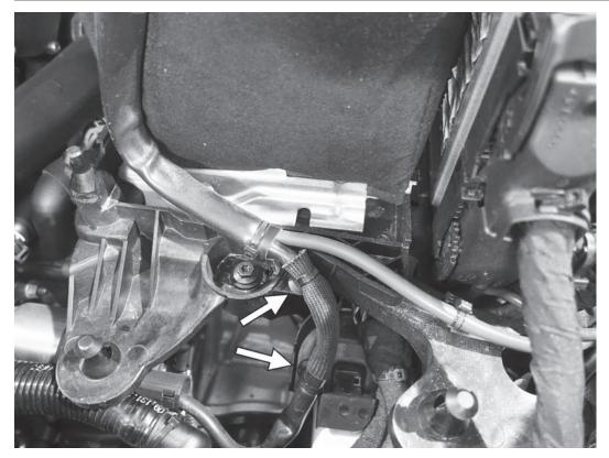
5) Cut and remove the two cable ties holding the battery cable to the bottom of the battery box. Remove the cable tie mounts from the battery box mounting points.
