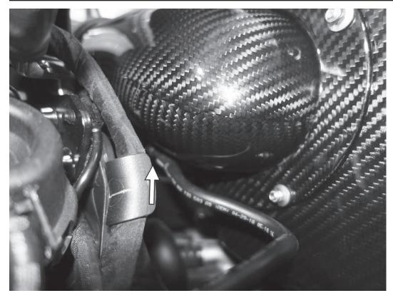
11) Connect the vacuum line that was on the right side of the factory airbox to the vacuum port on the bottom of the APR intake tube.
