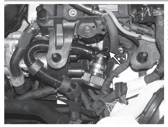
7) If equipped with Secondary Air Injection, install the secondary air filer (CI100020-A, sold separately) on the car. Snap the secondary air filter to the factory fitting on the secondary air pipe. Bend the pipe down to tuck it out of the way and secure it with a cable tie.
