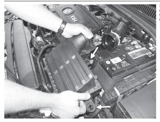
3) Firmly lift up on the back and side of the factory airbox, separating it from the two rubber mounts on the left and back sides of the airbox.
