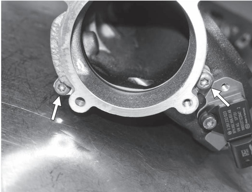
17) As viewed from where the throttle body mounted, remove the two T30 screws that hold the factory spacer to the upper intake manifold.
