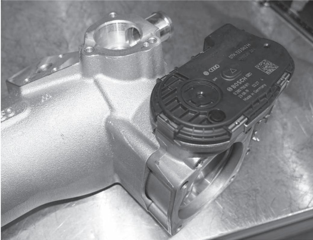
23) After lubricating the o-ring that was just installed, install the throttle body to the APR cast inlet pipe, noting the orientation of the throttle body motor to the diverter valve flange on the casting.
