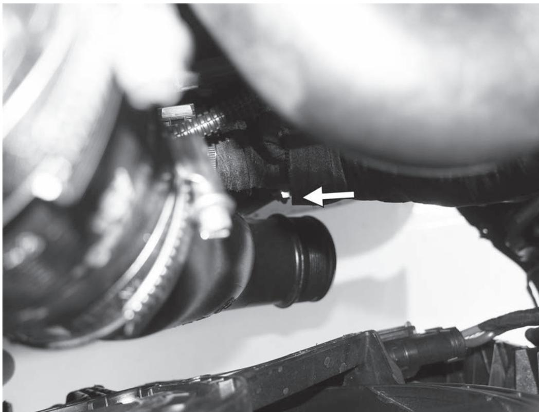
11) On the factory intake tube leading into the factory intake pipe, locate and remove the 10mm screw holding the tube to the engine. Remove the factory intake tube from the car.
