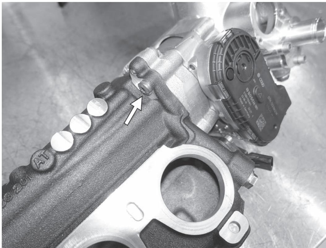
13) On the back side of the upper manifold assembly, remove the T30 screw holding the throttle body to the intake manifold.
