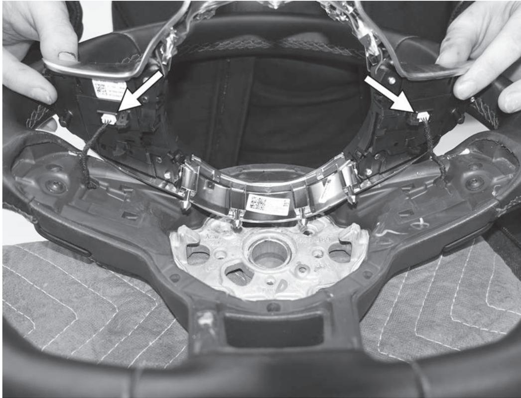
17) On DSG cars, once the trim is fully separated from the steering wheel, disconnect the two electrical connectors that go from the DSG paddles to the back of the multifunction buttons.
