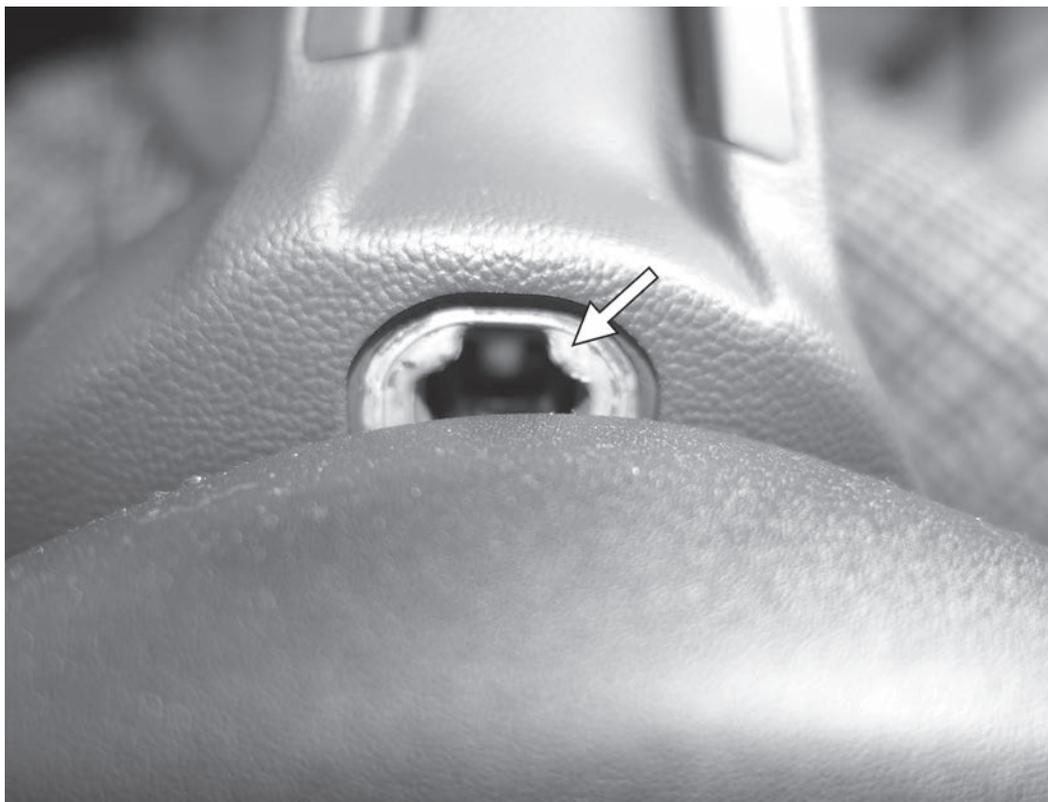
3) On the back side of the steering wheel, on the left wheel spoke facing up, locate the metal slot.
