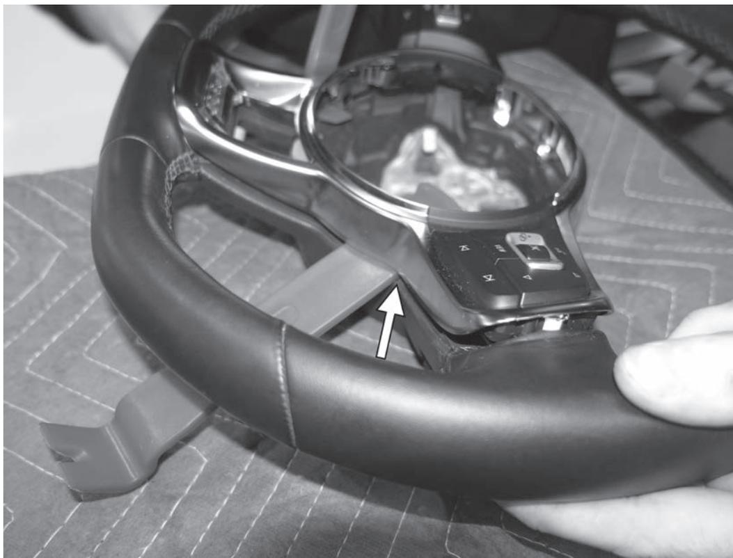
15) Work your way to the bottom of the steering wheel, separating the trim piece from the steering wheel.
