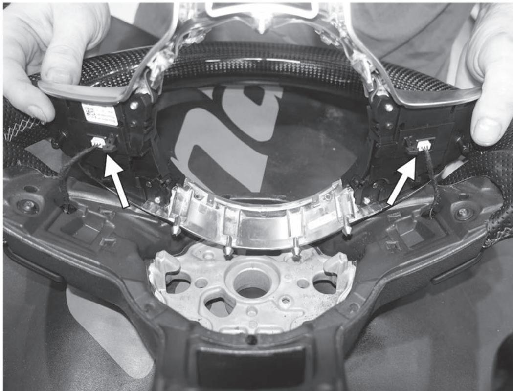
21) Connect the wires from the DSG paddles to the back of the steering wheel trim piece. Apply a lubricant that will evaporate (water or alcohol based) into all the holes the steering wheel trim will mount into.
