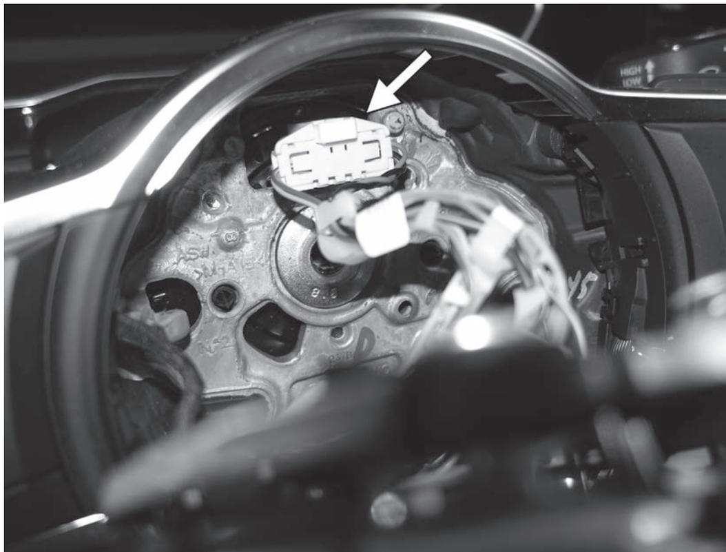
7) Pull the airbag away from the steering wheel. Disconnect the wiring harness to the airbag by pulling the white tab back away from the steering wheel, and then press down on the white tab to release the electrical connector.
