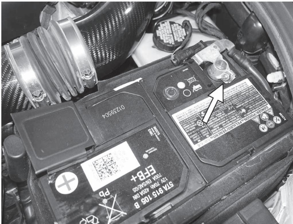
27) Reconnect the negative battery terminal to the car, and tighten the 10mm nut to 9Nm (80 in-lbs).
