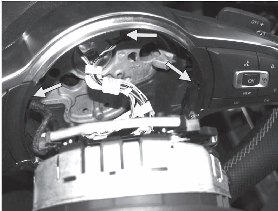
25) Place the airbag assembly close to the steering wheel. Reconnect the two smaller wiring harnesses to the sides of both the right and left wheel spokes, connecting the multifunction switches to the airbag assembly. Finally, reattach the connector for the main airbag wiring harness to the connector on the steering column. Be sure to push in the white tab on the connector to lock the connector in place.
