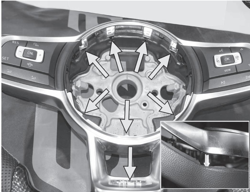
11) There are eight posts holding the plastic steering wheel trim to the steering wheel. The posts, shown in the inset picture, will all need to be separated in order to remove the trim. A fair amount of force is necessary, but be careful not to break them.
