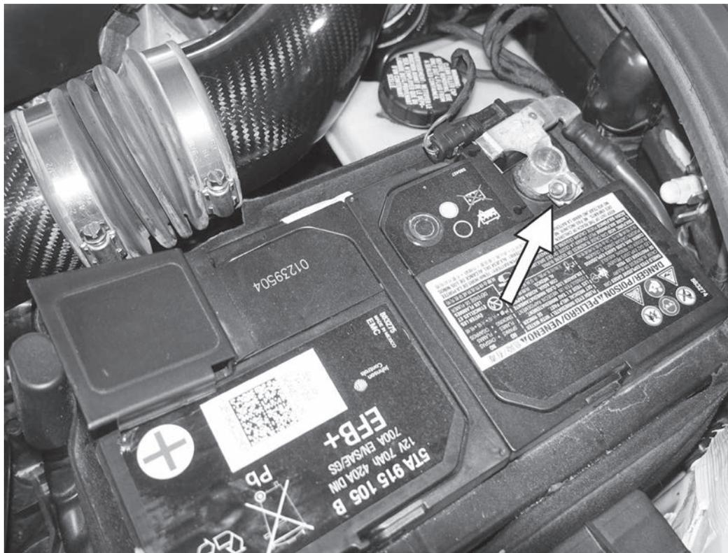
1) Disconnect the negative battery terminal by loosening the 10mm nut and lifting the battery cable off and away from the battery.
