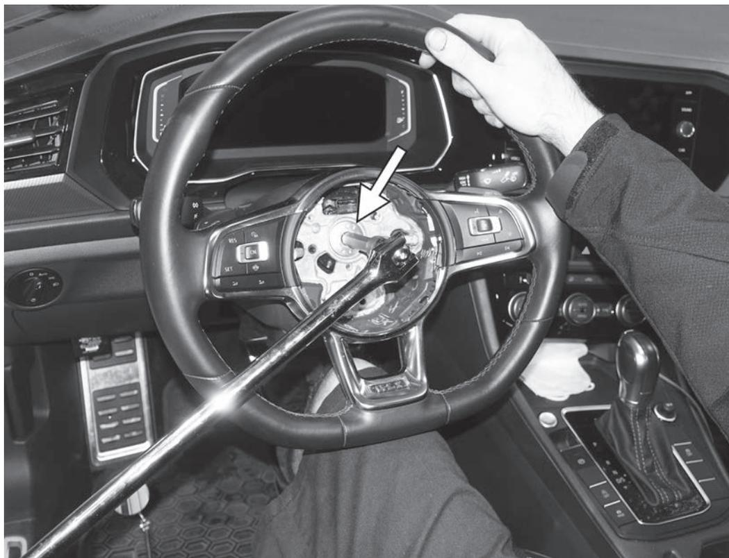
9) Using a 12mm triple square and a breaker bar, loosen and remove the bolt holding the steering wheel in place. Do not remove the steering wheel.
