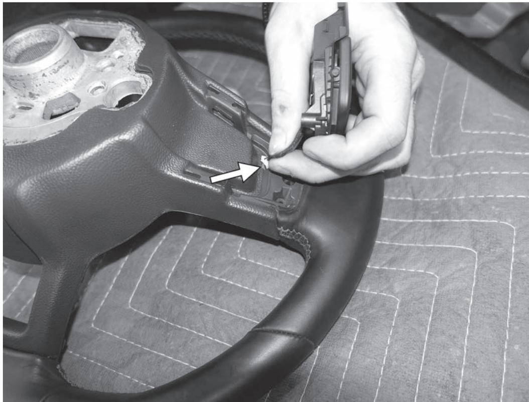
19) Remove the DSG paddles from the back of the steering wheel, and carefully pull the harness and connector through the steering wheel.
