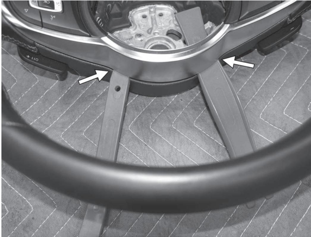
13) Continue working around the top of the trim, separating it from the back of the steering wheel. Use another trim tool to prevent the trim from snapping back onto the steering wheel.
