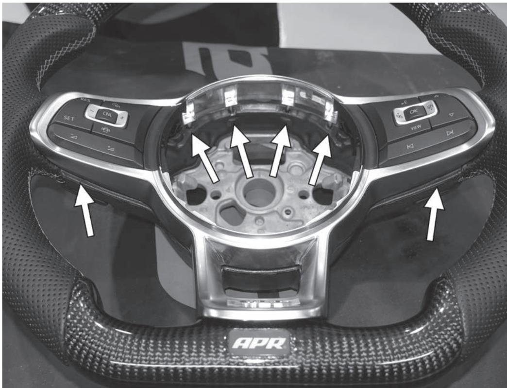
23) Work around the wheel from the bottom up, ensuring all the mounting posts are going into the correct mounting holes in the steering wheel.
