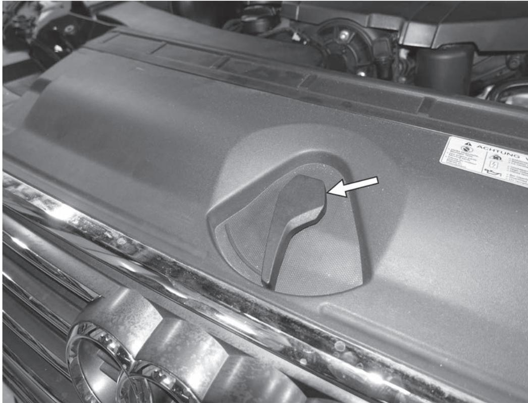
17) Reinstall the hood latch. The latch is keyed so that it can be only installed in one direction. Push the latch down until it clips fully onto the hood latch post.
