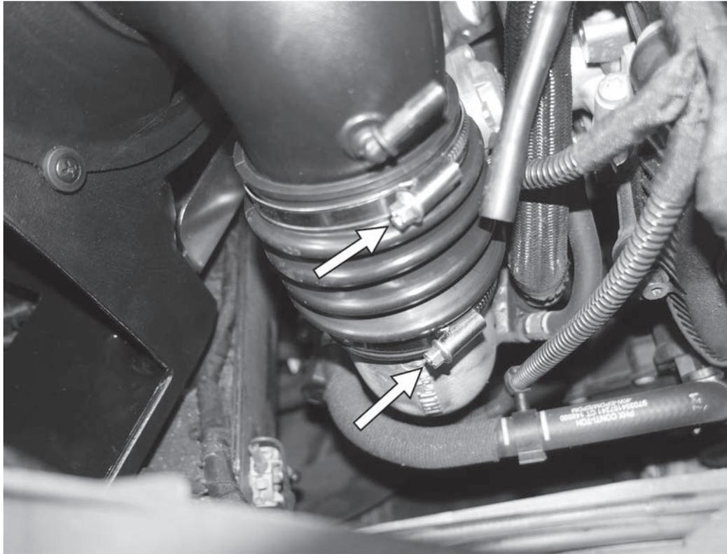
11) Ensure the coupler is correctly over the outlet of the airbox and the inlet of the turbocharger. Position the clamps as show, between the turbo inlet and the side of the engine, and tighten the both clamps to 5.5Nm (48in-lbs).
