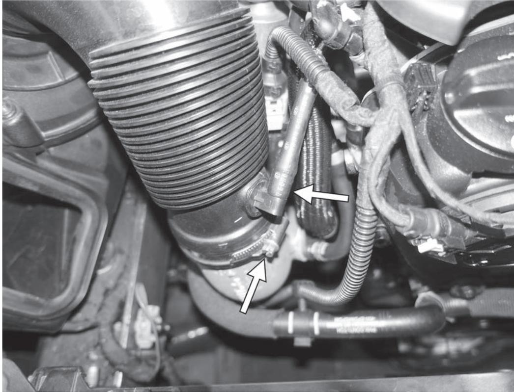
5) Pull off the rubber vacuum line from the plastic 90° fitting on the front of the turbo inlet hose. Loosen the 7mm hose clamp connecting the turbo inlet hose to the turbocharger.
