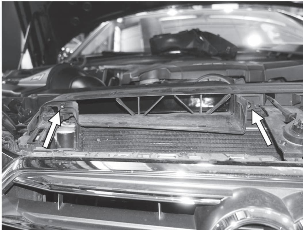
15) Install the two supplied 5mm allen screws from the front side of the core support and into the threaded mounting holes of the APR inlet scoop. Tighten the screws to 2.5Nm (22in-lbs).
