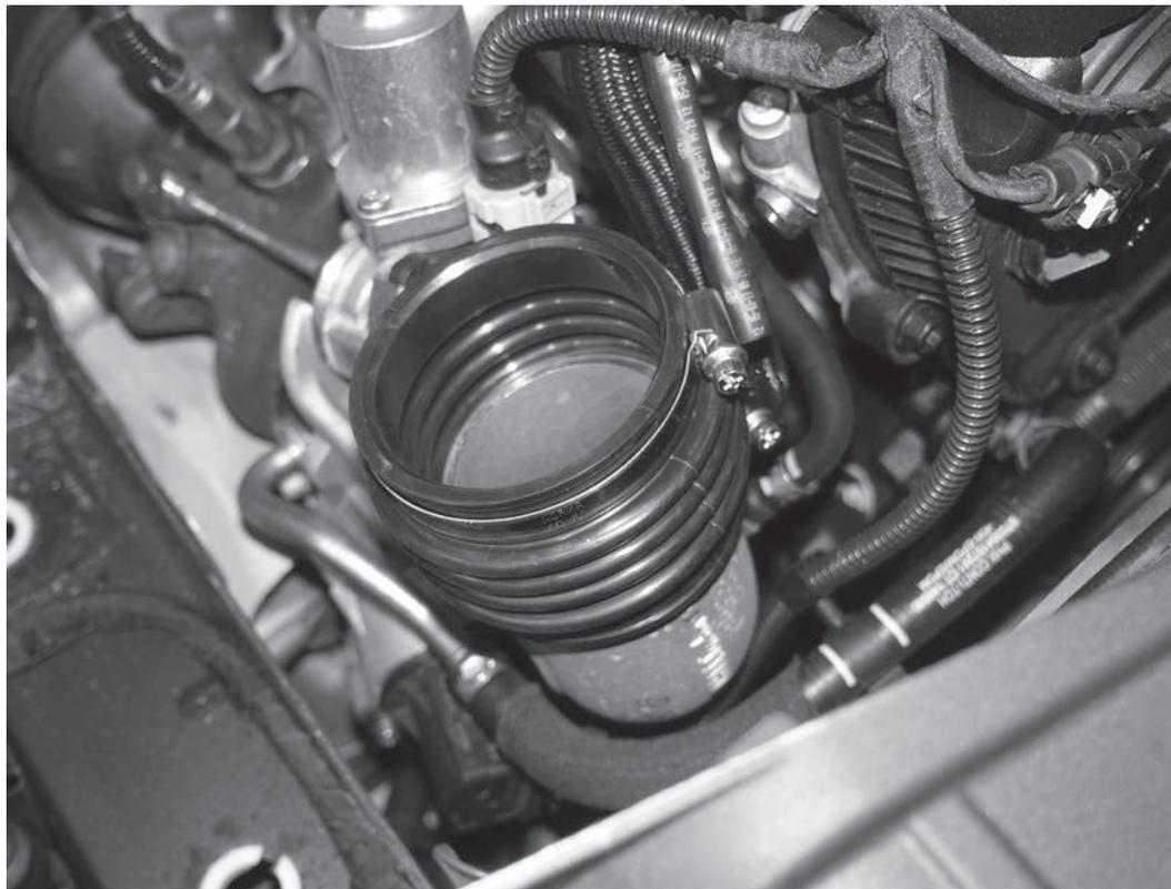
9) Install the APR coupler onto the turbo inlet pipe.
