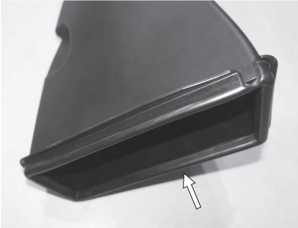
13) Install the rubber seal onto the end of the APR inlet scoop that goes into the APR airbox. The seal wraps around both the inside and outside of the inlet scoop.
