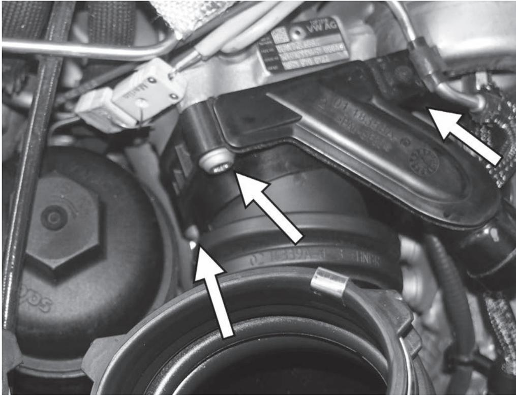
17) Remove the three T30 screws holding the left inlet flange to the left turbos.
