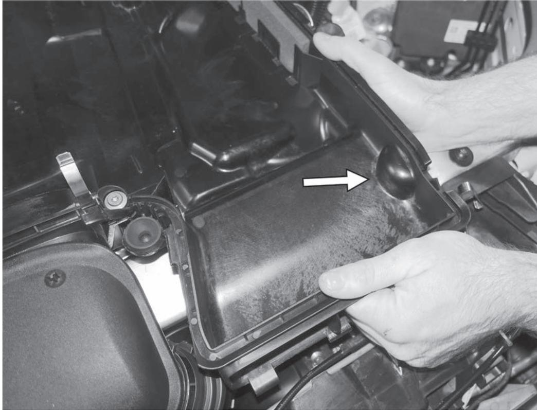
9) Lift up on both front corners of the airbox base to separate them from their mounting points. Do not yank on the cover, as you can break the back mounting points of the airbox base.
