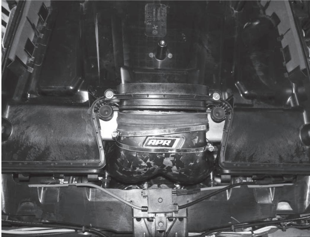
33) Place the factory airbox base back onto the engine by first attaching to the mounting points on the front of the firewall, then swing the front down and onto its original mounting posts.
