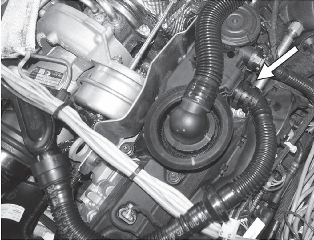
13) Unplug the front PCV connector from the left side of the engine, just behind the oil fill tube. Press in on both sides of the connector and pull away from the engine.
