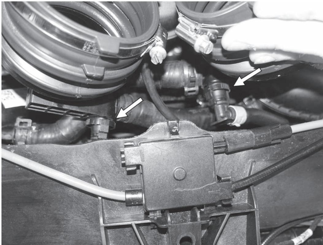
15) Disconnect the two quick disconnect fittings on the front of each front turbo inlet hose.
