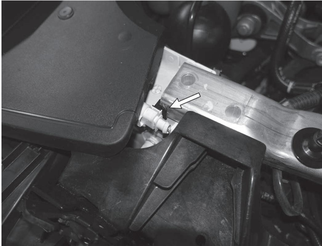
29) Reattach the crash sensor electrical connector to the right side of the front crossbrace, making sure to not unplug the electrical connector.
