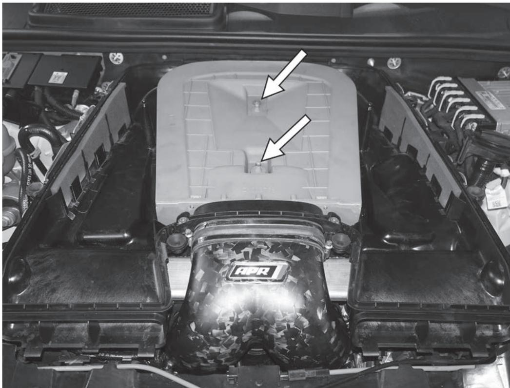
35) Install the APR air filter and secure with the two factory T25 screws and tighten to 5Nm (44 in-lbs).
