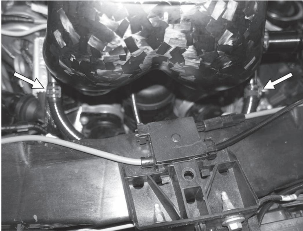
27) Connect the lines from the APR hose assemblies onto the ports on the front of the turbo inlet pipe. Adjust the routing of the hoses so that there are no kinks in the hoses. The hoses will cross from side to side; the hose assembly from the right side of the engine connects to the left port on the turbo inlet pipe, and the hose from the left side of the engine connects to the right port on the turbo inlet pipe.
