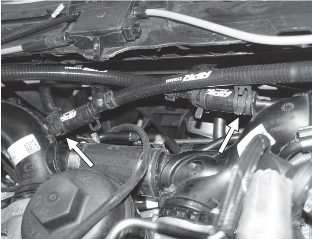
23) Install the APR hose assemblies to the connecting points the OEM hoses were attached to. Secure with the spring clamps on the APR hose assemblies.
