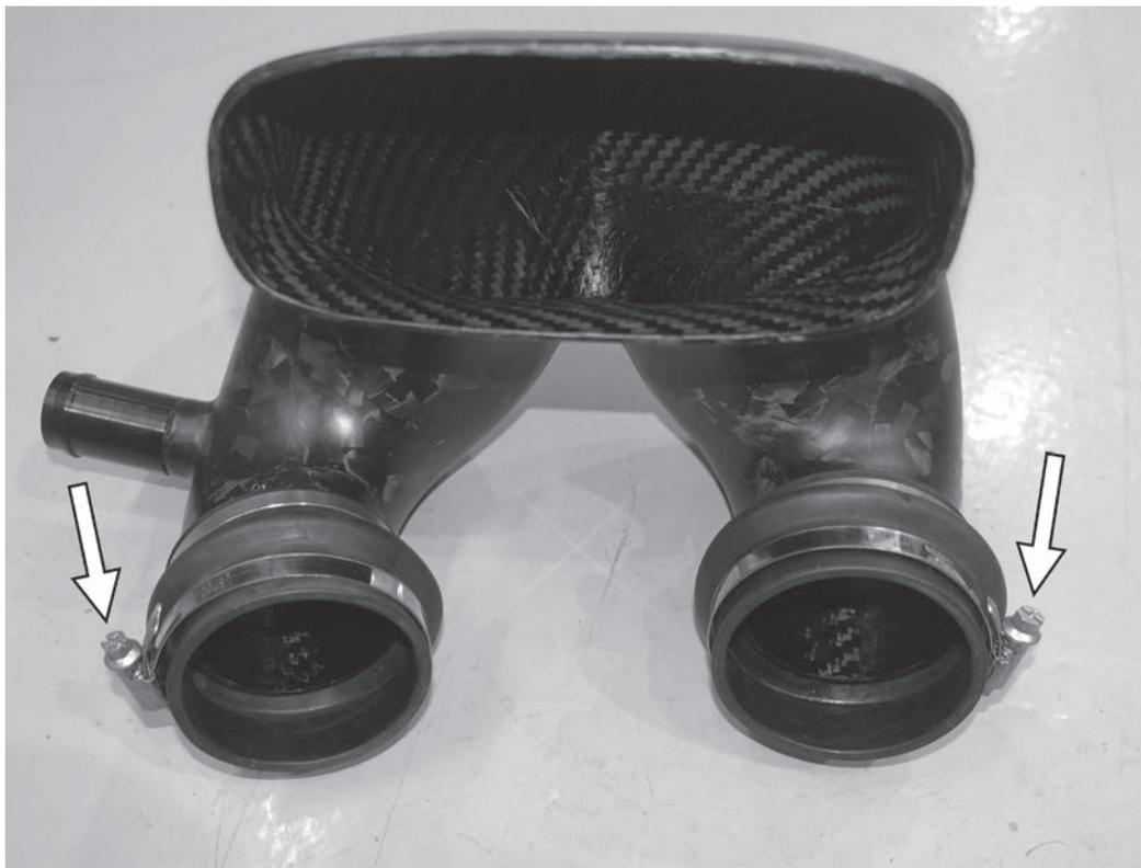
25) Loosely install the two screw clamps as shown onto the APR turbo inlet pipe.
