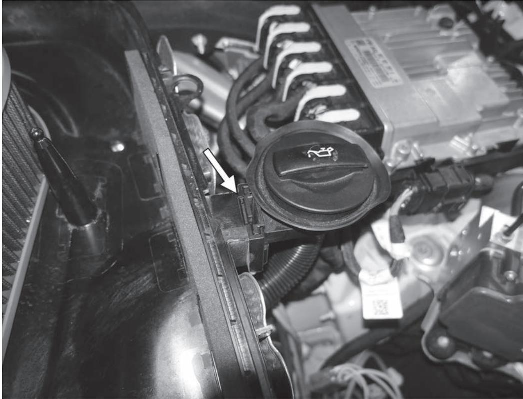
39) Reconnect the oil fill tube and cap assembly to the left side of the airbox base. Clip the tube assembly back into its original mounting location. Remove the oil fill cap.
