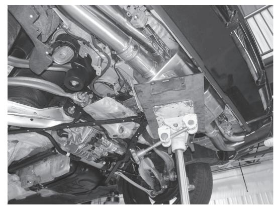
41) With an assistant, raise the APR muffler assembly into place, making sure muffler outlets sit inside the exhaust tips. Use a transmission jack to support the exhaust in place.
