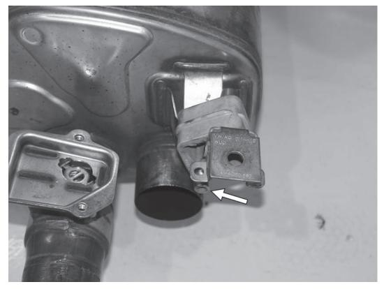
37) Remove both rubber exhaust hangers with their brackets from the factory exhaust, noting their orientation.
