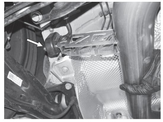
9) Place the APR bent pipe assembly onto the car. Push the longer bracket into the previously installed rubber exhaust bushing on the rear subframe.
