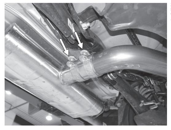
21) Adjust the sleeve clamp just before the rear muffler, and then tighten the two 15mm nuts to 20Nm (177 in-lbs).
