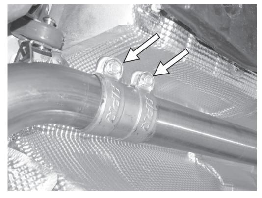
19) Adjust the sleeve clamp at the back of the center exhaust tunnel, and then tighten the two 15mm nuts to 20Nm (177 in-lbs).
