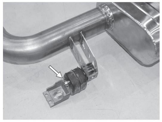
7) Remove the rubber hangers with exhaust brackets from the stock rear muffler section. Install the mounts on the APR rear muffler in the same orientation as on the stock exhaust, with the hanger side away from the muffler.
