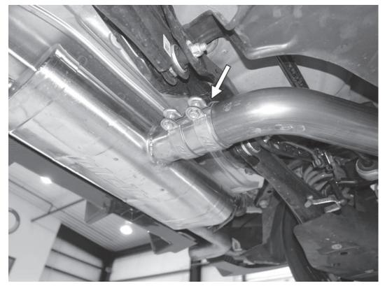
11) Connect the back of the APR bent pipe assembly to the APR rear muffler assembly with one of the supplied sleeve clamps. The clamp can be loosely tightened, but still needs to be adjusted.
