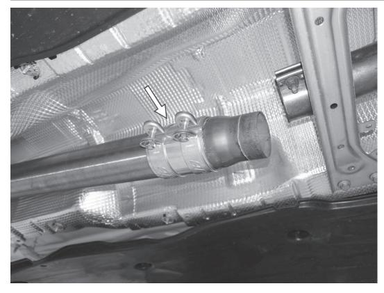
13) On the front side of the straight section of pipe, install the supplied reducer with the last supplied sleeve clamp. The clamp can be loosely tightened, but still needs to be adjusted.
