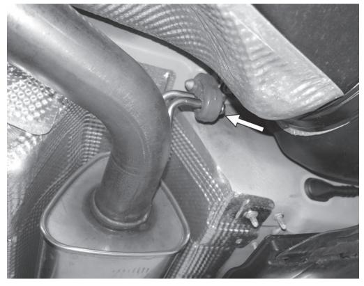
5) Separate the stock exhaust from the rubber exhaust bushing near the back of the center tunnel of the car. Leave the rubber bushing attached to the car. Lower the entire rear section of the exhaust and remove it from the car.
