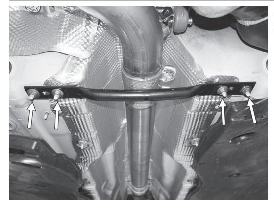
15) Reinstall the rear crossbrace on the car with the four original 13mm nuts. Tighten the nuts to 20Nm (177 in-lbs).
