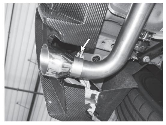
17) Loosely install the two rear exhaust tips with the two 13mm band clamps. The clamp can be loosely tightened, but still needs to be adjusted.
