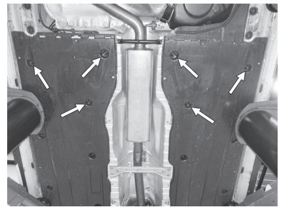
1) Securely place the car on a lift or jackstands. Remove six 10mm nuts from the back of each side underbody panel, three on each side.
