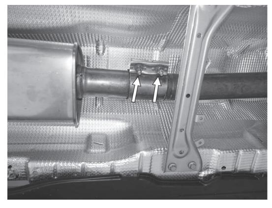
3) Loosen the two 13mm nuts on the factory sleeve clamp, just behind the front crossbrace.
