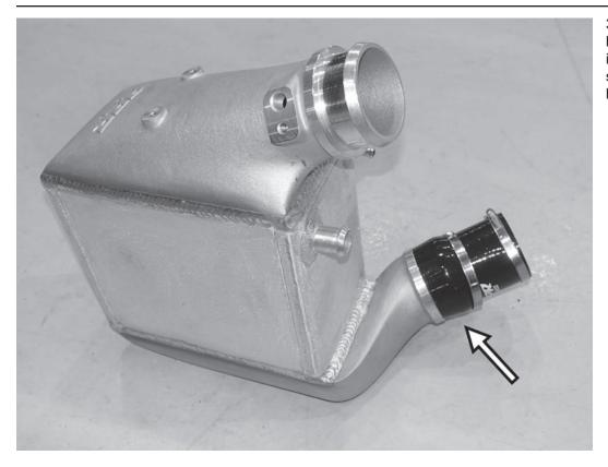
39) Install the APR lower intercooler hose (Z1003822) loosely onto the inlet of the APR intercooler. Loosely secure the hose with the supplied hose clamp.
