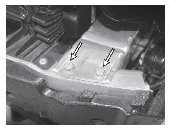
59) Push the bumper crash beam back in place. A deadblow hammer may be needed to push the crash beam back to its original mounting points. Install the four 13mm screws and nuts holding the crash beam in place, and tighten them to 23Nm (17ft-lbs).
