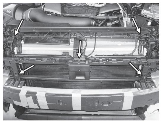
17) Remove the five T30 screws holding the upper bumper support to the radiator core support.
