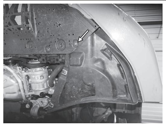
69) Reinstall the two front wheel spoilers and secure with the T25 screw from underneath. Reattach the headlight drain lines to the back side of the spoiler.
