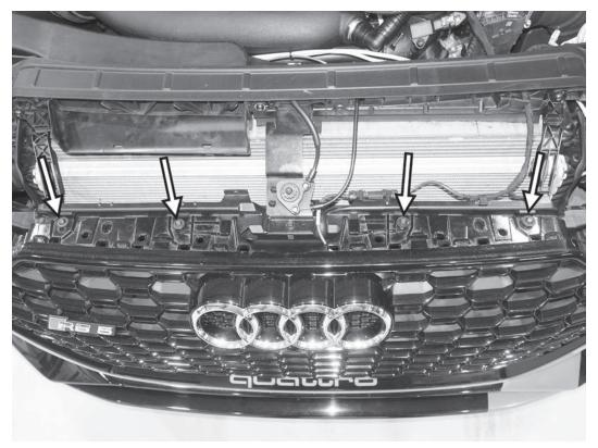
5) Remove the four T30 screws holding the top of the bumper cover to the upper bumper support.
