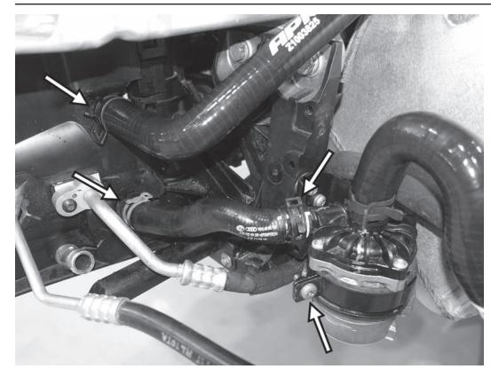
49) Reconnect the factory coolant hose to the side of the coolant pump, and then to the connection by the radiator support and secure with the spring clamps. Connect the other end of the previously installed APR hose (Z1003825) to the top connection of the front radiator and secure with a spring clamp. Finally, when the factory coolant hose is without tension, fully tighten the T30 screw on the coolant pump bracket to 9Nm (80in-lbs).
