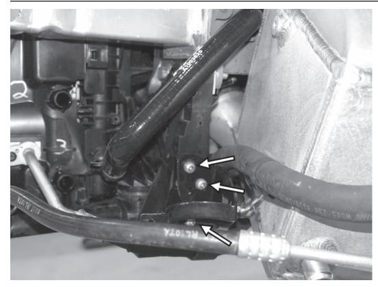
43) Reinstall the stock auxillary coolant pump bracket in its original location, sandwiching the APR lower intercooler bracket between the pump bracket and the radiator core support. Loosely install the three original T30 screws. Tighten the three upper 5mm APR intercooler mounting bracket screws to 9Nm (80in-lbs). The tighten the three factory T30 screws on the coolant pump bracket to 9Nm (80in-lbs). Finally, tighten the 10mm hex screw on the lower APR intercooler bracket to 9Nm (80in-lbs).
