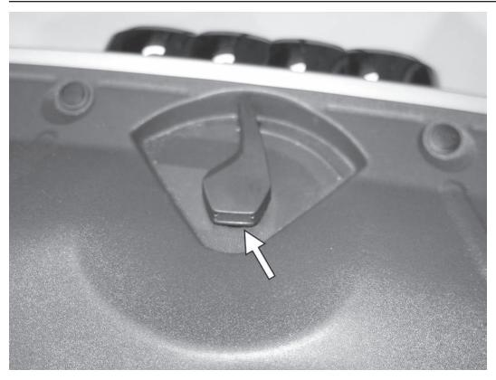
75) Reinstall the hood release latch. The latch is keyed, so it can only go on in one position.
