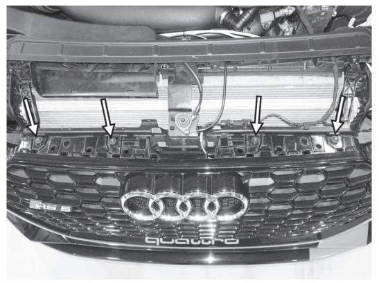
67) Reinstall the four T30 screws along the top of the bumper cover to the upper bumper support.
