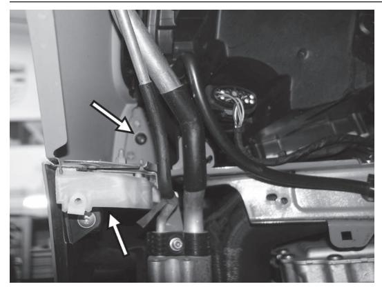
9) Remove the T30 screws holding the bumper cover to the front side of the fender. Also remove the push pin style connector between the side of the bumper cover and the bottom of the front fender. Repeat on the other side of the car.
