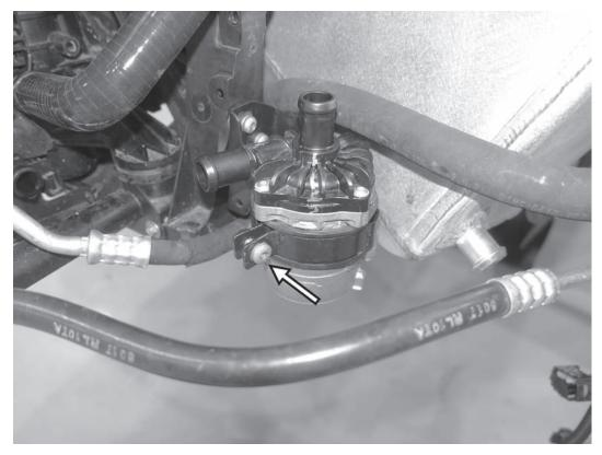
47) Reinstall the factory coolant pump with the original T30 screw. Leave the screw loose, so the pump can be rotated if necessary.
