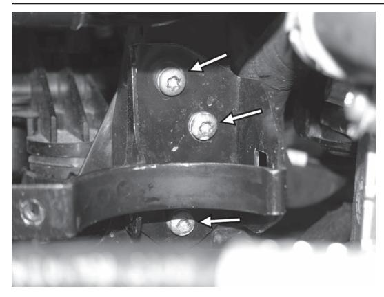
33) Remove the three T30 screws holding the auxillary coolant pump bracket to the side of the radiator support, and remove the bracket from the car.
