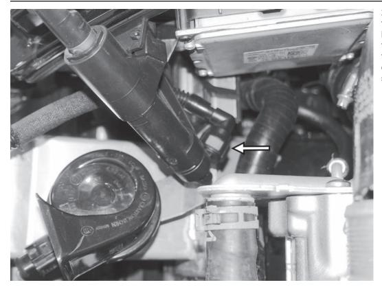
21) Disconnect the washer fluid line from behind the back of the left headlight washer by pressing on the blue tab. Also disconnect the washer line that is on the right side of the bumper crash beam. The washer line will stay attached to the crash beam.
