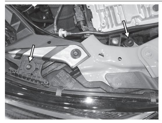
25) Remove the last two T30 screws from the top of the left headlight, and then carefully slide the headlight forward to remove it from the car. Place the headlight somewhere that it cannot be damaged.
