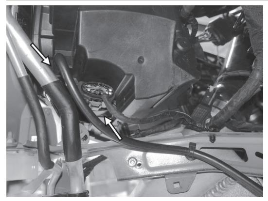
55) On the back side of the headlight, reconnect the drain hose and the electrical connector to the headlight.
