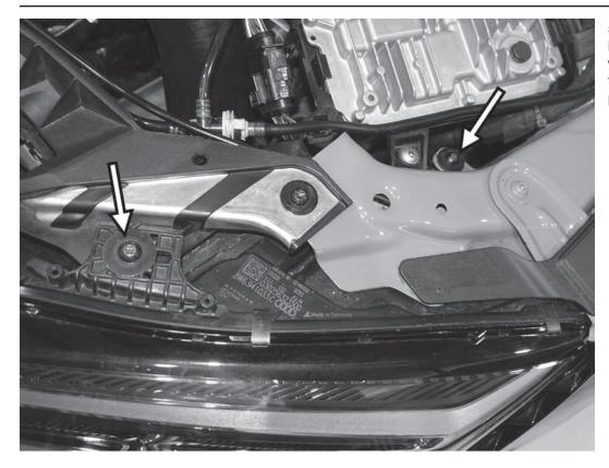
53) Carefully slide the left headlight back in place, and loosely secure it with the two original T30 screws. Try to align the headlight in its original position.
