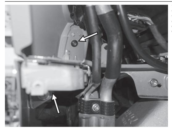
71) Reinstall the T30 screws holding the bumper cover to the front side of the fender. Install the push pin style connectors that go between the side of the bumper cover and the bottom of the front fenders.
