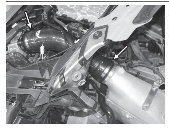
45) Install the APR upper intercooler hose (Z1003821) between the throttle body and the APR intercooler outlet. Tighten the hose clamps to 3.4Nm (44in-lbs). Also position and tighten the two clamps on the lower APR intercooler inlet hose to 3.4Nm (44in-lbs).
