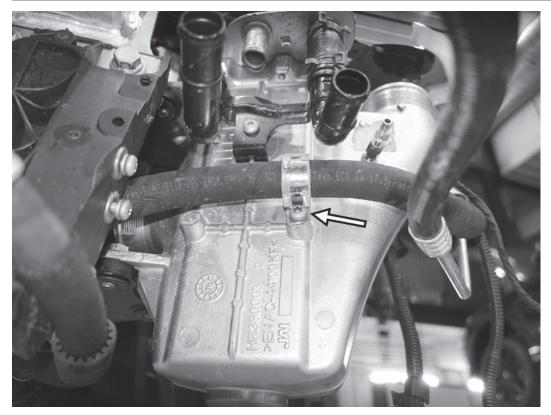
35) Remove the T30 screw holding the air conditioning line from the front of the stock intercooler. Remove the bracket from the AC line as well.
