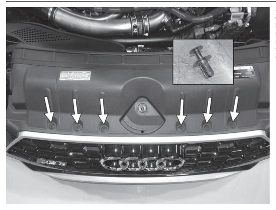
3) Remove the six push pin style connectors holding the cover between the front bumper and the radiator support. Carefully pry the raised center part of the pin up, and then remove the entire pin assembly up and out of the cover.
