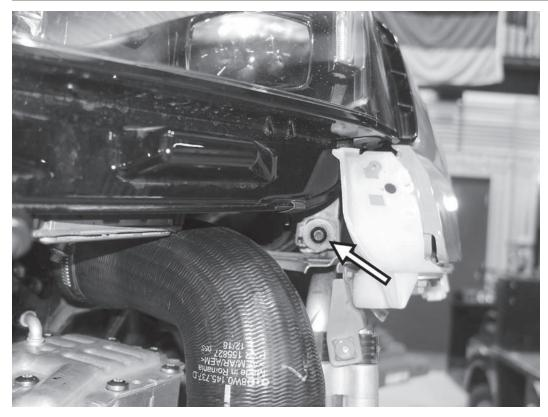
23) Remove the T30 screw from underneath the left headlight, by the front fender.
