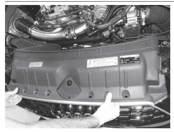
73) Place the upper bumper cover back on the car. Place the back side of the cover into the radiator core support, and then lower the front side of the cover behind the front grille.
