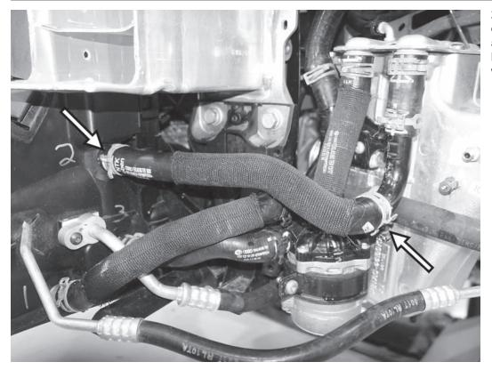
29) Loosen the two spring clamps on the coolant hose on the top of the auxillary radiator, and remove the hose from the car. Be aware coolant will spill as these hoses are removed.
