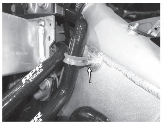
51) Install the rubber clamp on this final coolant hose (Z1003826), and secure to the top boss on the front of the APR intercooler with one of the 5mm allen screws with a flat washer. Tighten the screw to 9Nm (80in-lbs).
