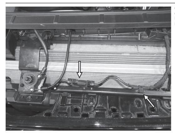
65) Reconnect the cable to the front distance sensor, and reattach the harness to the upper bumper support.
