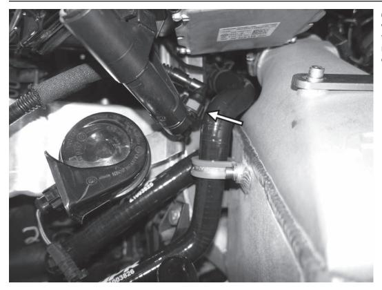
63) Reconnect the windshield washer line from the crash beam to the left headlight washer. Also reconnect the windshield washer line on the right side of the crash beam.
