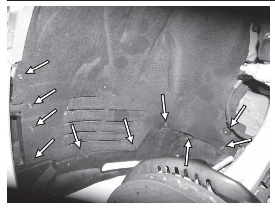
7) Remove all the fasteners from the front side of the wheel well liner. Typically, this is ten T25 fasteners, two 10mm nuts, and one T30 screw. Repeat this step on both sides of the car.
