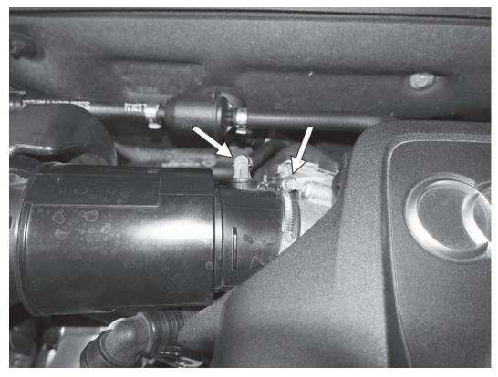
1) Raise the hood on the car, and then loosen the hose clamp on the back side of the accordian intake tube at the throttle body. Disconnect the vacuum line from the back of the intake tube by the throttle body.
