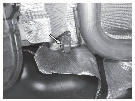
5) At the back of the center tunnel of the car, separate the exhaust from the rubber exhaust hanger, leaving the rubber hanger attached to the car.
