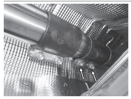
11) After flipping the factory sleeve clamp around, install the assembled section of pipe onto the back of the factory exhaust. After leaving approximately a 10mm gap between the sections, loosely tighten the 13mm nuts on the factory sleeve clamp to hold the straight assembly on the car.
