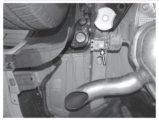
7) With an assistant holding the factory muffler up, remove the two 13mm bolts on both sides of the rear muffler. The entire factory exhaust can then be lowered down from the car once it is slid out of the previously loosened sleeve clamp.
