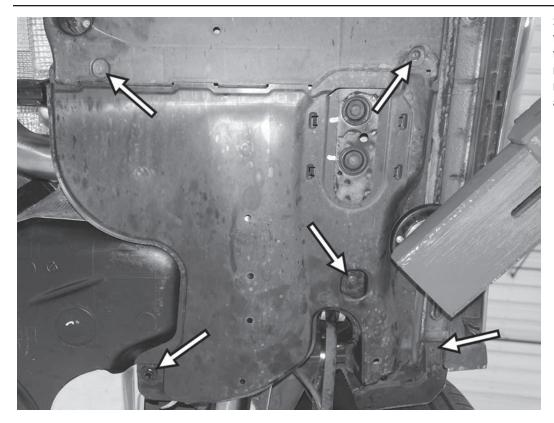
3) From the underbody panel just in front of the left rear wheel, remove the four T25 screws and one 10mm nut holding the panel in place. After noting how the tabs on the panel is attached, remove it from the car.
