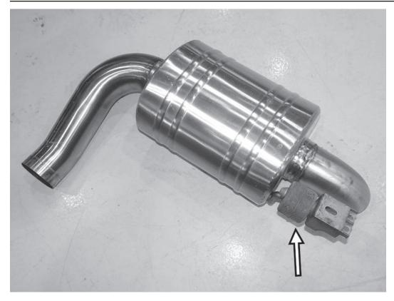
9) Install the factory exhaust hanger assembly onto the APR rear muffler in the same orientation.
