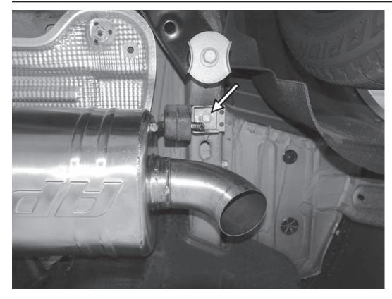
17) Tighten the 13mm screw on the rear muffler hanger to 20Nm (15ft-lbs).
