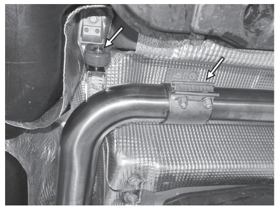
13) With an assistant, install the center section of the APR exhaust to the car to the factory rubber hanger at the back of the center tunnel. Loosely install one of the APR sleeve clamps to hold the center section of the exhaust to the previously installed straight section of the exhaust.
