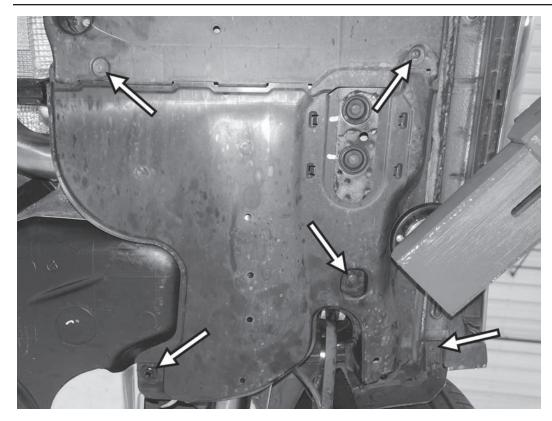
19) Reinstall the underbody panel just in front of the left rear wheel, making sure the tabs on the panel go back in the same way it was removed. Install the four T25 screws and one 10mm nut holding the panel in place, tightening all fasteners to 2Nm (18in-lbs)
