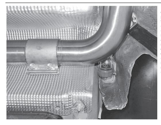
15) Working from the front of the exhaust to the back, adjust the position of the exhaust and tighten the sleeve clamps. The exhaust (cold) should hang slightly forward (towards the front of the car) on the rubber hanger. There should be approximately 10mm between each section of pipe inside the sleeve clamps. Tighten the two 13mm nuts on the factory sleeve clamp to 30Nm (22ft-lbs). Tighten the four 15mm nuts on both sleeve clamps on the straight section of exhaust to 61Nm (45ft-lbs).
