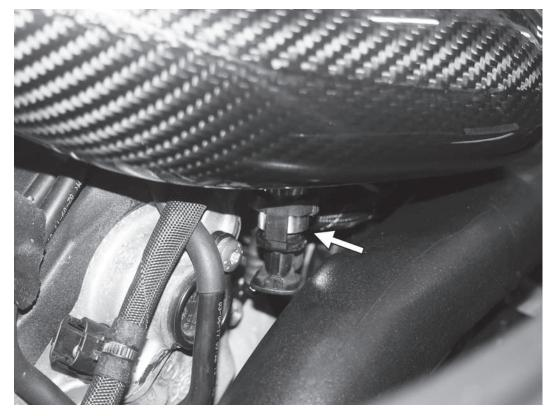
9) Slightly lift up on the turbo inlet pipe, and then disconnect the hose connection from the bottom of it by squeezing on both sides of the connector. Remove the turbo inlet pipe with silicone couplers and clamps from the car.
