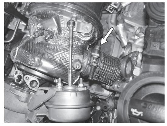
33) Loosen the 10mm triple square from the v-band clamp holding the exhaust coupler to the turbo. Separate the clamp so it is free.
