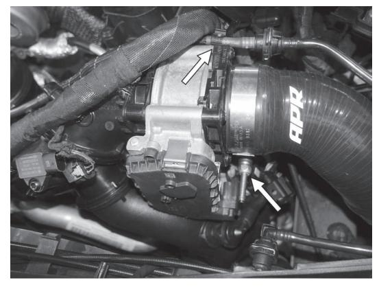
63) Reattach the charge pipe to the throttle body, and tighten to 5.7Nm (50 in-lbs). Reconnect the coolant line behind the throttle body to the clip on the back of the throttle body.
