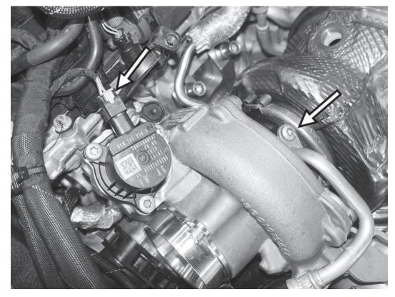
21) Disconnect the electrical connector on the diverter valve. Slide the grey locking tab back first, before squeezing the connector to unplug it. Remove the T30 screw from the oil feed line on the top of the turbocharger.
