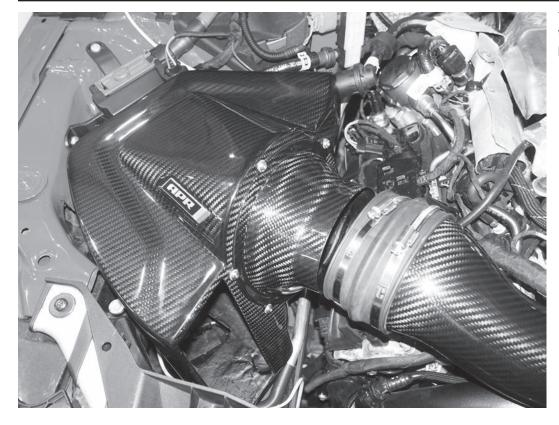
71) Reinstall the airbox assembly in the car. and reconnect the turbo inlet pipe to the airbox.
