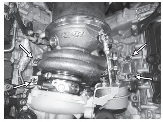
45) Install the four supplied 10mm triple square copper nuts to hold the turbo in place. Tighten all four nuts in a crossing pattern to 15Nm (11 ft-lbs). Then, tighten all four nuts again in a crossing pattern to 30Nm (22 ft-lbs). Finally, check all four nuts to ensure they are at 30Nm (22 ft-lbs).
