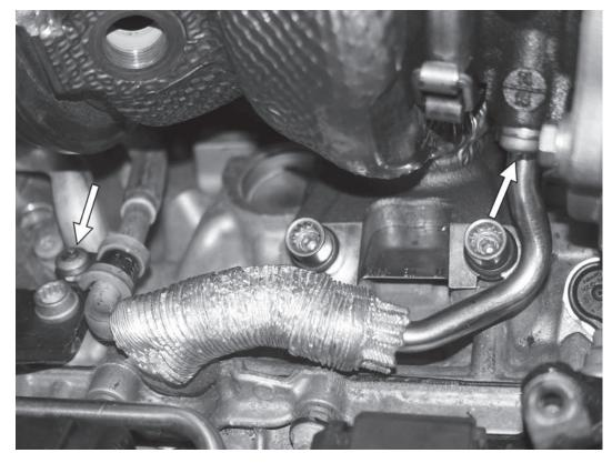
31) Remove the T30 screw from the coolant feed line on the right side of the turbo. Remove the T30 screw holding the coolant feed line to the right cylinder head, and then separate the coolant feed line from the turbo.
