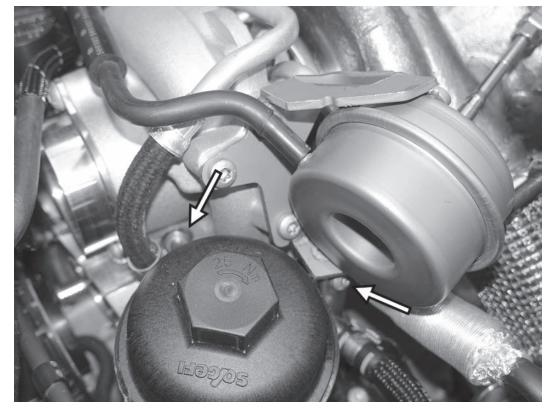
55) Route the hard vacuum line under the wastegate actuator as it was on the stock turbo, and then stick the vacuum line in the hole just behind the compressor inlet. Install the T30 screw into the bracket on the hard vacuum line and secure the line to the side of the turbo. Tighten the screw to 9Nm (80 in-lbs).
