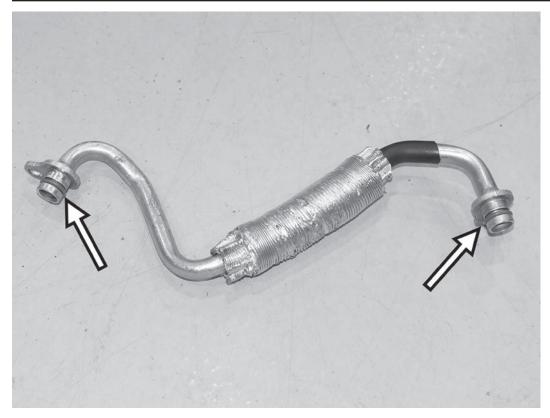
41) Remove the coolant line from the side of the stock turbo. Remove and replace the two o-rings with two of the supplied green o-rings.
