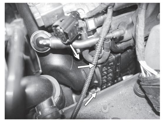
25) Unscrew the three T30 screws holding the charge pipe to the left intake manifold.
