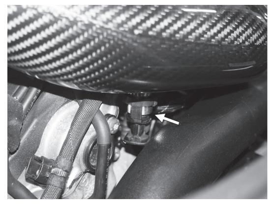
69) Slightly lift up on the turbo inlet pipe, and then connect the hose connection to the bottom of the turbo inlet pipe.
