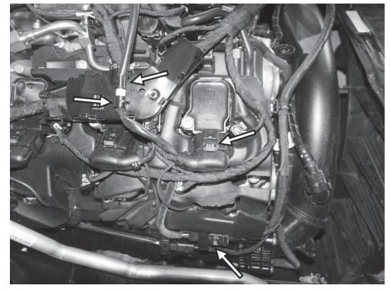
57) Reroute the oxygen sensor harness down the right side of the engine, reconnecting the harness to the clips on the side of the engine. Route the harness underneath the wiring harness as before, and then reconnect the oxygen sensor harness to the main harness. Reattach the electrical connector to the bracket on the side of the engine.
