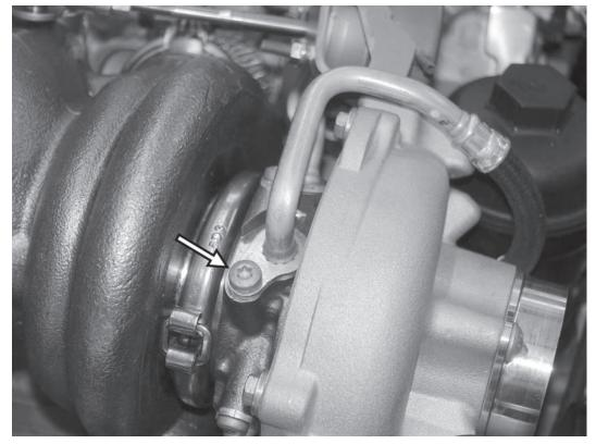
51) Replace the o-ring on the oil feed line with another one of the green o-rings, and then install the oil feed line to the turbocharger. Tighten the screw to 9Nm (80 in-lbs). Connect the electrical connector to the diverter valve on top of the turbo.
