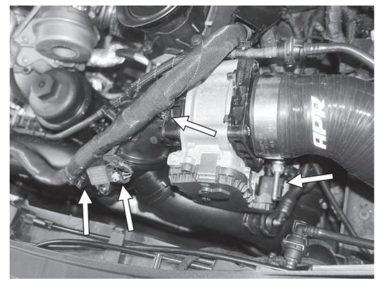
23) Unplug the electrical connectors from the throttle body and from the MAP sensor to the right of the throttle body. Separate the wiring harness clip from the front charge pipe and on top of the throttle body.
