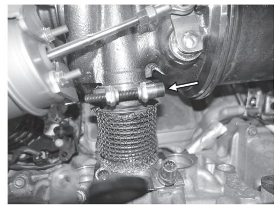
47) Once seated correctly, tighten the 10mm triple square on the exhaust coupler to 20Nm (177 in-lbs).
