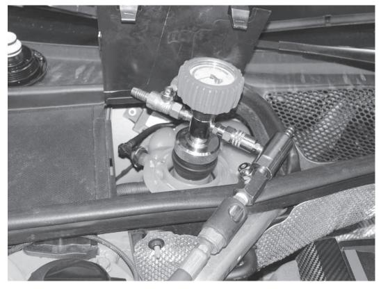
75) Refill the engine coolant using a vacuum bleeder style system. Follow the tool manufacturers instructions for vacuuming and refilling the engine coolant. Fill with new engine oil if the oil was drained.
