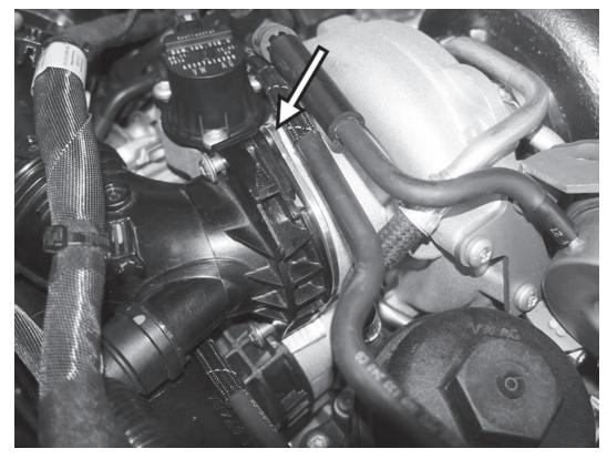
67) Place the stock inlet adapter onto the captive screws on the stock inlet pipe, with the o-ring groove facing the turbo. Carefully place the pipe onto the front of the turbo, ensuring the o-ring stays in place and the raised lip of the adapter goes into the inlet of the turbo. Tighten the two T30 screws to 9Nm (80 in-lbs).
