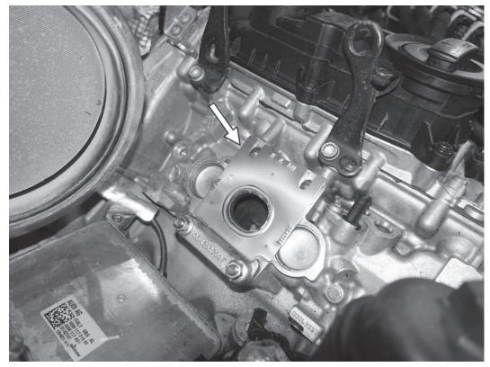
35) Be careful not to drop anything into the engine (the exhaust ports, oil drain hole, or coolant drain hole), covering the openings with a rag as necessary. Remove the old exhaust gaskets from both the right and left exhaust ports on the cylinder heads. Clean up the gasket mating surface if needed. Set the new gaskets in the slot on the lower bracket, the same way they were when they were removed.
