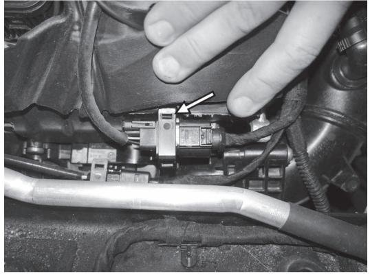
13) Unclip the oxygen sensor connector from the bracket, and disconnect the connector from the wiring harness. Route the oxygen sensor harness out from behind the ignition coil harness to completely free the oxygen sensor harness from the car.
