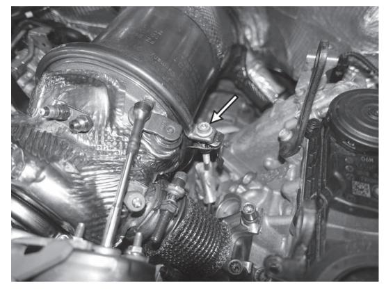
17) Loosen the 6mm allen screw (or T30 screw) on the v-band clamp holding the downpipe to the turbo. Once loose, pry up on the clamp and slide it to the back of the catalyst.
