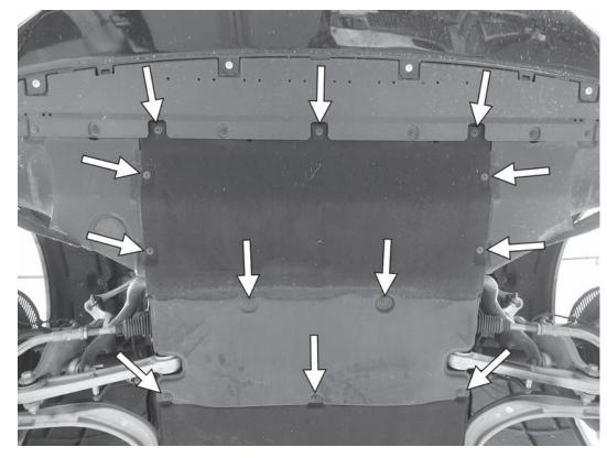
15) Loosen the coolant cap from the coolant expansion tank under the cowl cover. Raise the vehicle and remove the twelve T25 screws holding the center belly pan to the bottom of the car, and then remove the belly pan. Note the way the belly pan is attached to the other panels around it, including the bottom of the front bumper cover.
