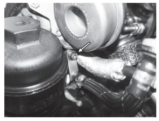
19) Just behind the oil filter housing, remove T30 screw holding the vacuum line that goes into the compressor housing of the turbo.
