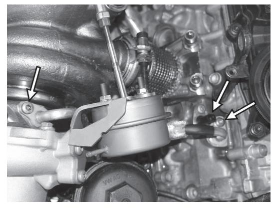
49) Install the coolant line on the left side of the turbo, in the same routing as it was stock. Install the two correct T30 screws and tighten to 9Nm (80 in-lbs). Reconnect the electrical connector to the coolant temperature sensor.
