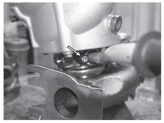
37) Lubricate both sides of the new, supplied oil drain line with clean engine oil. Install the oil drain line in the turbo with the previously removed factory plastic press-in plug. If the plastic plug breaks, a 5MM allen screw can be used to hold the oil drain line in place. This fastener is only used to hold the oil drain line in place while it is being installed, so it can be very lightly fastened.
