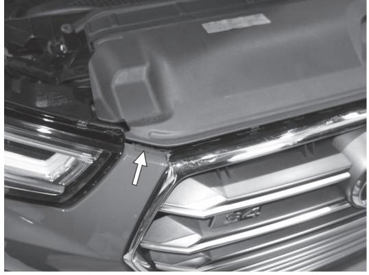
73) Place the back of the hood latch cover into the slot of the radiator support. Then, carefully align the tabs along the front of the hood latch cover and snap them back into their correct positions along the top of the bumper and grill.
