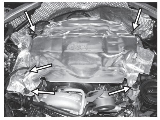
65) Reattach the factory heat shield to the top of the engine with the four 13mm mounting posts. Tighten the mounting posts to 5Nm (44 in-lbs). Reattach the clip on the oxygen sensor harness to the heat shield. Reinstall the engine cover on the engine.
