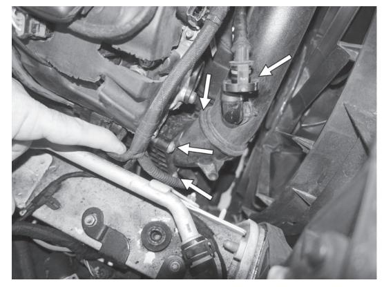
61) Loosely reinstall the three T30 screws that hold the front charge pipe to the right intake manifold. Try to rethread the screws in the original holes, as the self tapping screws can otherwise strip the intake manifolds. Reinstall the Norma style connection to the port on the intake charge pipe. Reclip the wiring harness onto the bottom of the front charge pipe.
