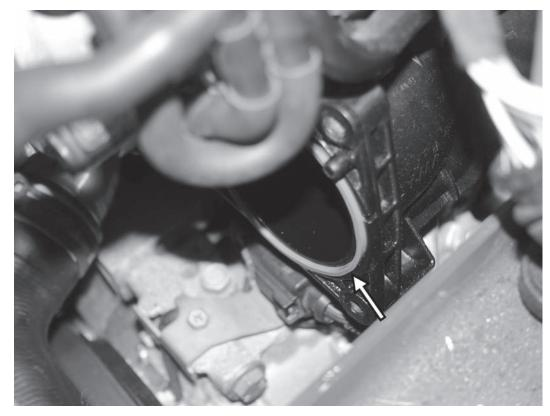
59) On the front charge pipe, remove both rubber gaskets from both inlets to the intake manifolds. Replace the gaskets with the new, supplied gaskets.
