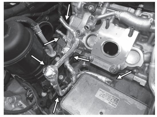
43) Using the supplied adhesive heat shielding, wrap the three vacuum lines with check valves in front of the oil cooler and behind the oil filter. Some lines can be wrapped by running the adhesive tape down the length of the hose and then wrapping it around, other areas will need to be spiral wrapped in the heat shielding. It may be necessary to clean these lines with a solvent first, like brake parts cleaner, in order for the adhesive to properly stick to the lines.
