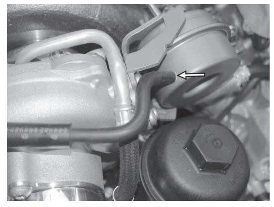
53) Swing the wastegate vacuum line and the hard vacuum line back over from the right side of the engine, and attach the rubber vacuum line to the wastegate on the APR turbo.
