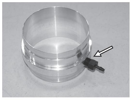
1) Securely screw the vacuum fitting into the side of the APR TSI inlet adapter.
